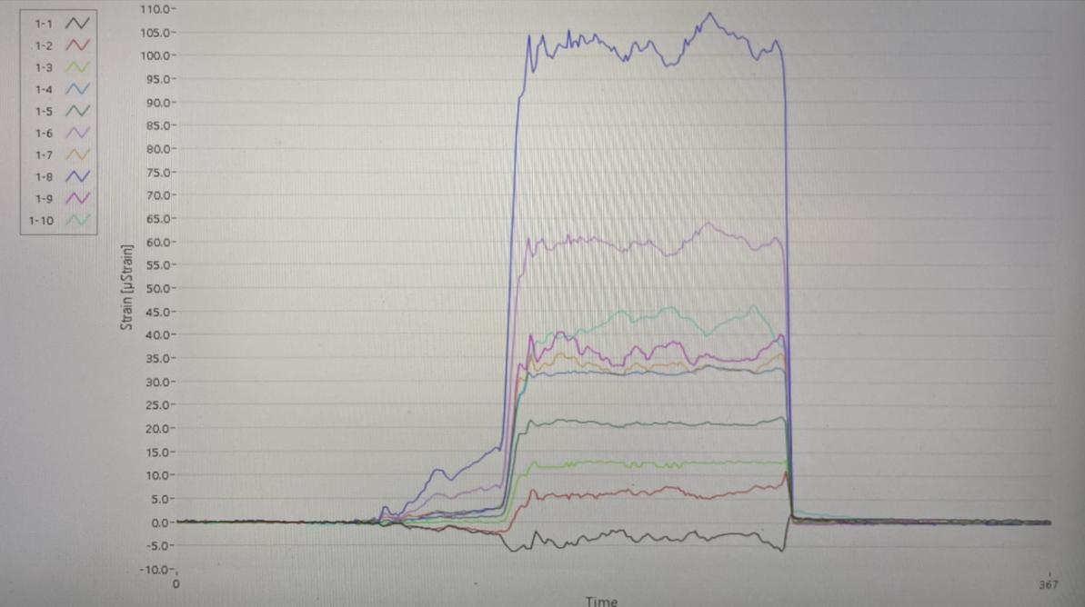
Figure 5.6: Example strain graph from 10 of the measurement points along the FBG strip as a result of loading the bridge by stepping onto the bridge, and stepping off again after a couple of seconds.
