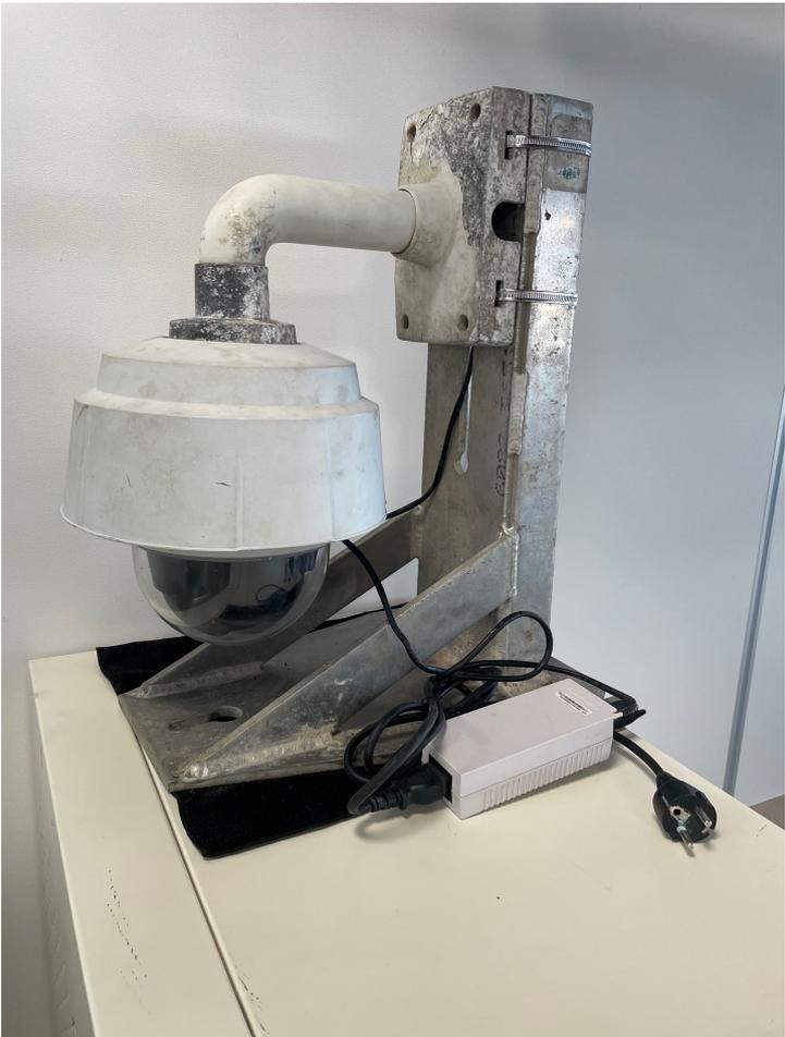
Figure 7.3: Axis Q6055-E Camera, as used in the experimental setup.
