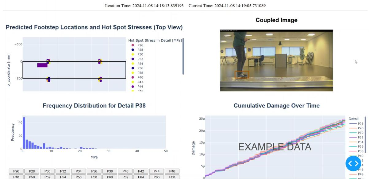
Figure 7.26: Screen capture of the dashboard during asset testing, displaying multiple useful views of the current state of the asset.
