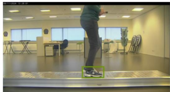
**Figure 7.13:** Experimental setup image from DAM3 for the single load case  $a = 1495$  mm,  $b = 300$  mm,  $F = 834$  N.
