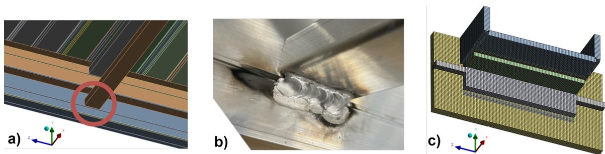
Figure 4.3: a) Global FEM model highlighting one sub-model (circled in red). b) Picture of the researched sub-model on the asset. c) Sub-model showing the adjusted weld plate thickness from the weld.
