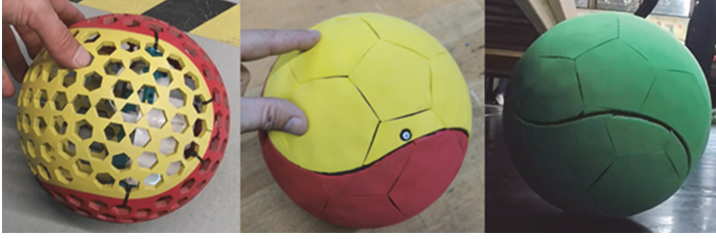
Fig. 2. Spherical robot prototypes used in the workshop (left and middle: LEGObased system, right: custom-designed system).
