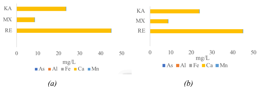
Figure 3.5 Average accumulated elements concentration in different types of studied water; (a) indicates the result with pipe sets 1, (b) indicates the result with pipe sets 2
