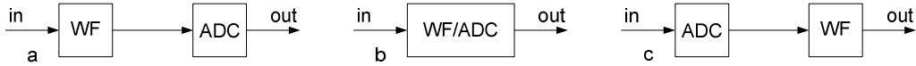
Figure 2.2. a: wavelet filter before ADC. b: wavelet filter inside ADC. c: wavelet filter after ADC
