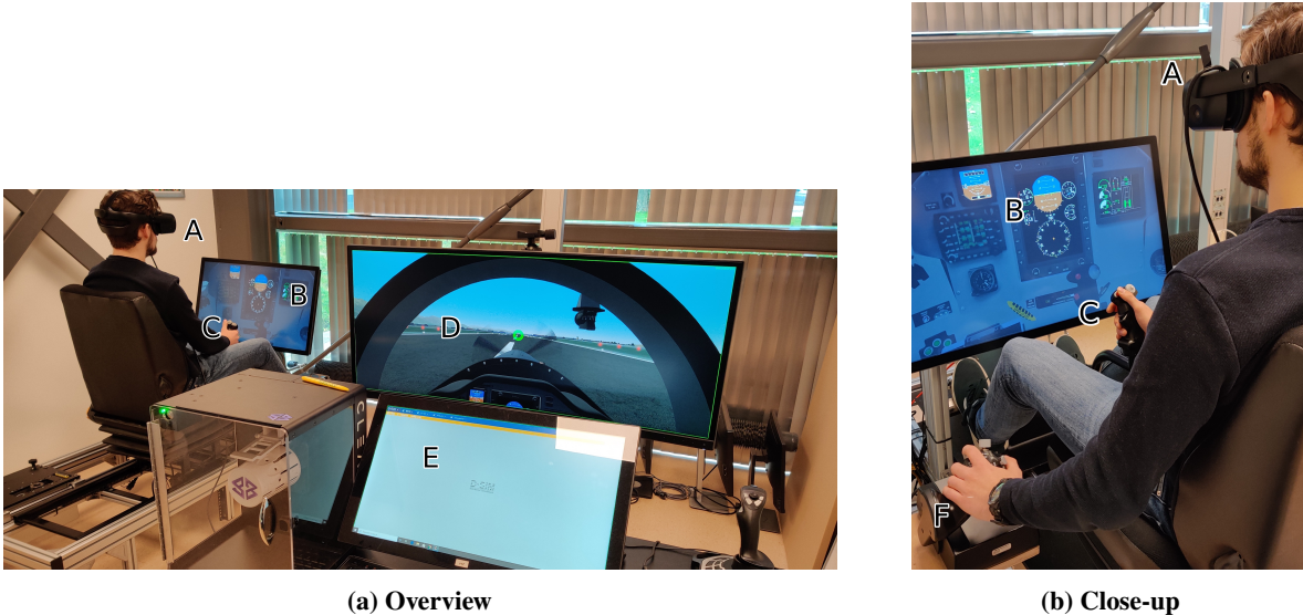
Fig. 3 Simulator setup during the experiment. A: VR headset, B: Cockpit instruments, C: Control stick, D: Participant's view, E: Instructor control panel, F: Throttle
