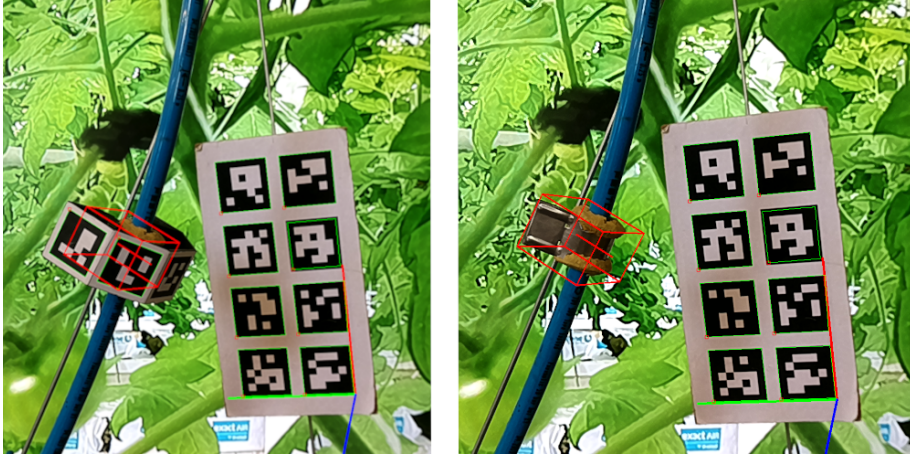
Figure 3.4: Aruco ring that is attached on the clip using magnets to register the relative transformation to the Aruco board. After this, the ring is removed. An annotation can then be created if the board is in view.
