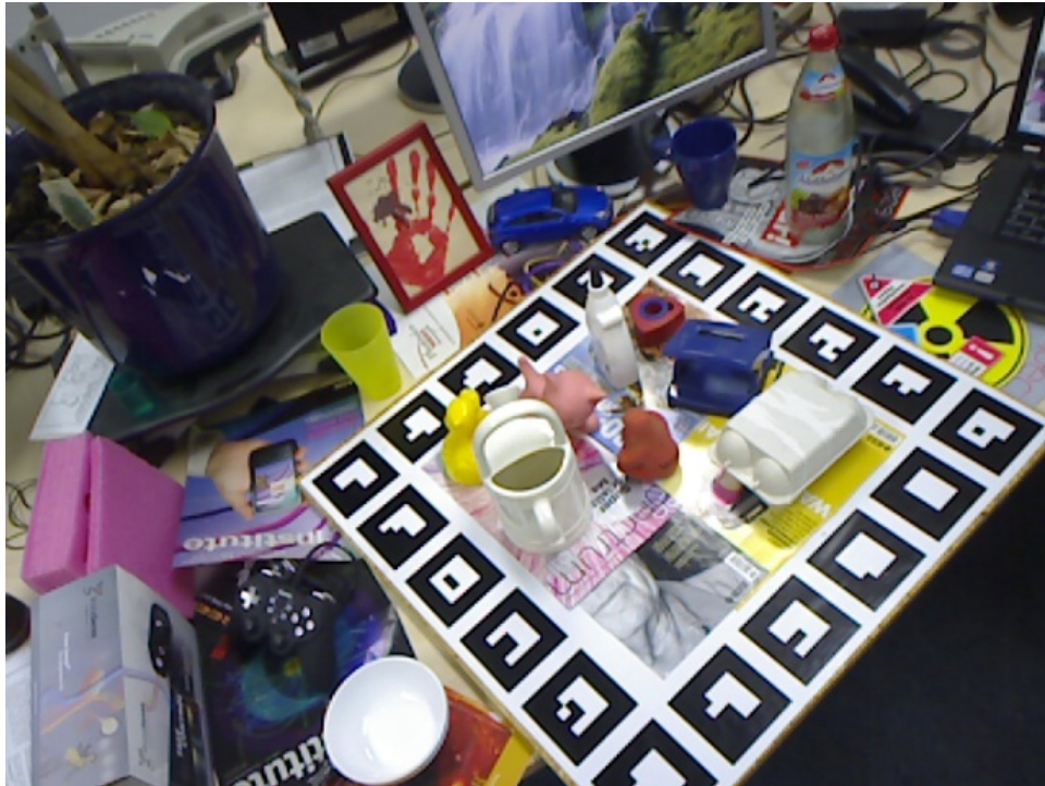
Figure 3.3: Items are placed randomly on a table with a surrounding ring of markers that register an object’s relative position for the LINEMOD dataset [12].
