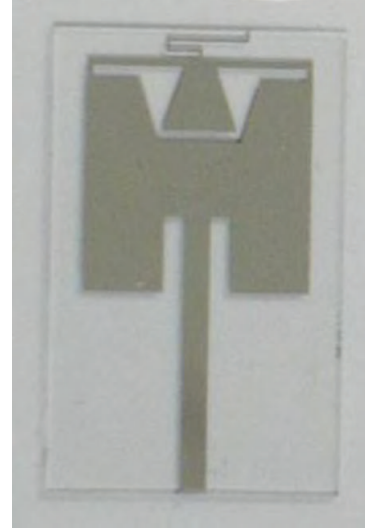
FIGURE 4: Frequency switchable antenna based on MEMS technology [7].
