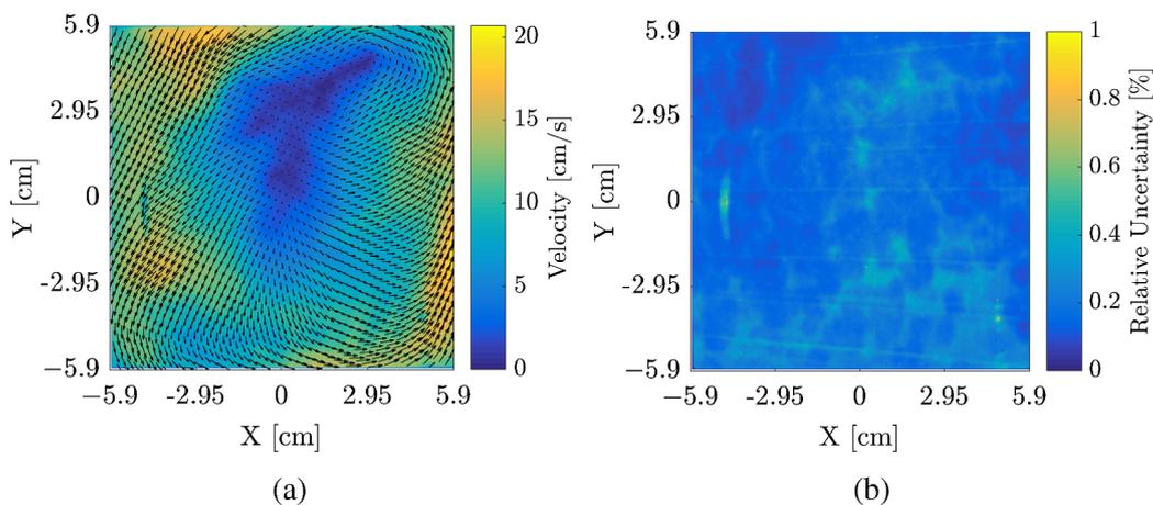
Fig. 4. Rotating at 2500 RPM (a) avg. vel. field (b) relative uncertainty.
