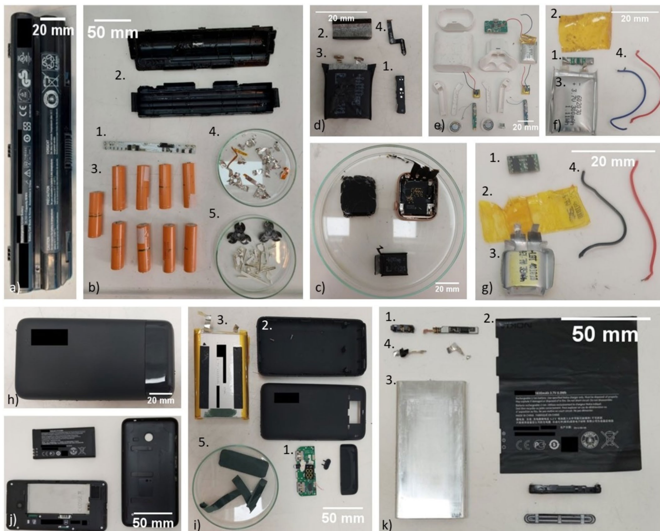
Figure 1. Battery modules (some of which with device) before and after disassembly. Represented are a (disassembled) laptop battery module (a, b), smart watch (c, d), set of wireless earphones (e, f, g), powerbank (h, i) and mobile phone module (j, k). For all sub images, the numbers represent the same component: 1. BMS, 2. Battery casing, 3. Battery cells, 4. Wiring, 5. Glue and separating components.
