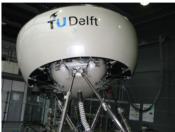
Figure 4.2: The SIMONA Research Simulator (Stroosma et al., 2003)
