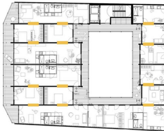
Figure 14: Removable walls in the typical floor plan (Analysis author: Ying Shen)
