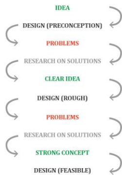
Fig. 5. From first idea to feasible design – design process
