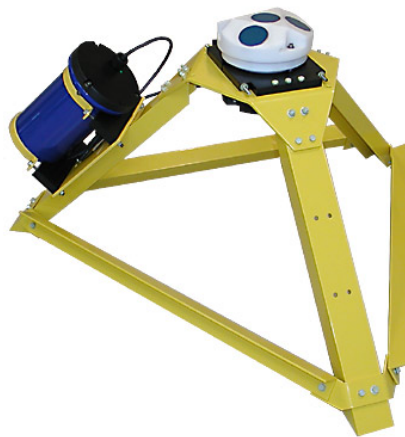
Figure D.1: Acoustic wave and current ADCP
