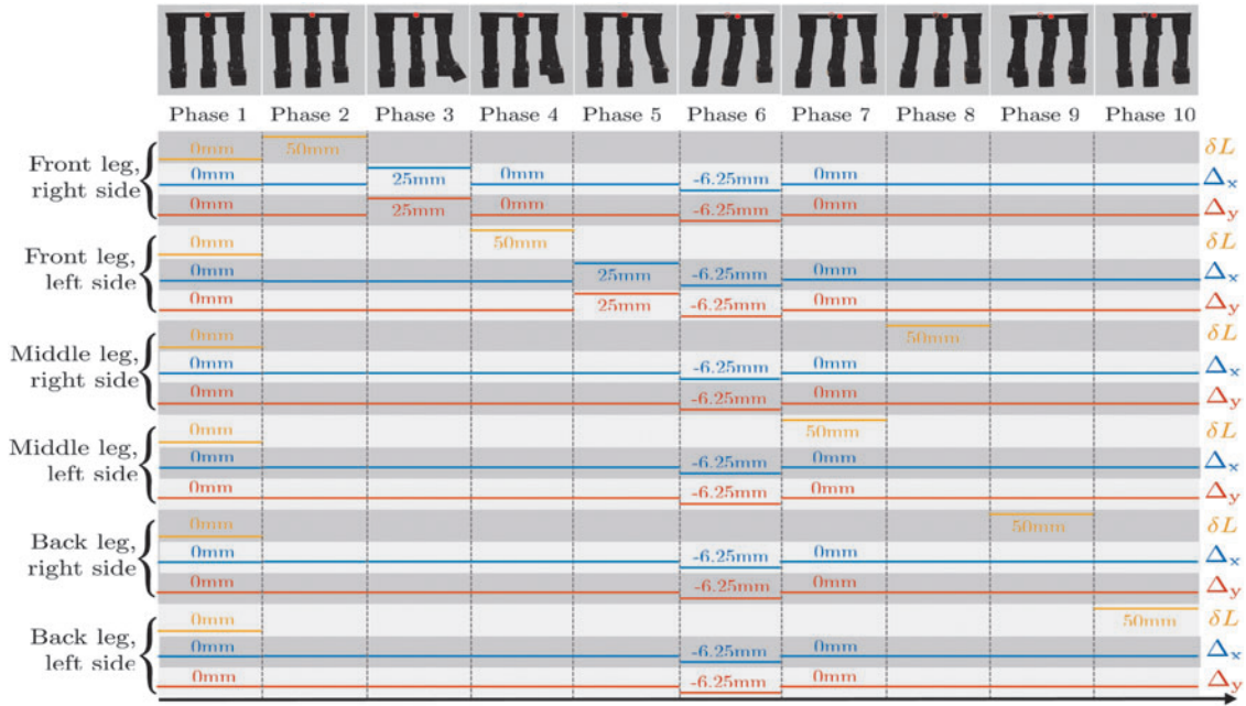
FIG. 5. Locomotion strategy and control for the large hexapod robot. Inspired by the locomotion of the octopus, the robot starts from a relaxed configuration (phase 1). The two front legs are then moved forward through a sequence of contraction, bending forward, and relaxing (phases 2 and 3 for the right leg, and phases 4 and 5 for the left). Subsequently, all six legs bend backward, pushing the robot's body forward (phase 6). Finally, the four back legs are sequentially contracted and relaxed so to put them in place (phases 7, 8, 9, and 10). The cycle then starts back from the beginning. Red dots indicate the evolution of the top sheet's center during locomotion (locomotion speed \approx 4.5 cm/min, gait cycle \approx 200 s).
