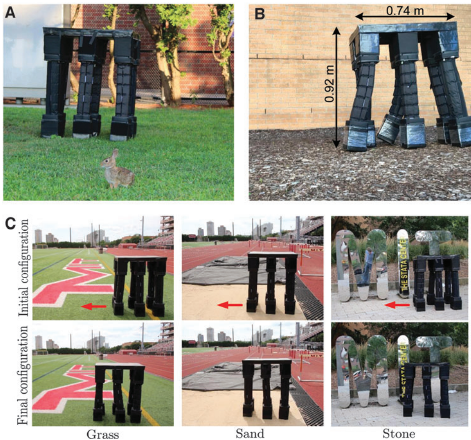
FIG. 4. Meter-scale untethered hexapod robot. (A, B) A large-scale legged soft robot, built using six soft modules as the legs and a sheet of foam as the body. We investigated the locomotion strategy for this large soft robot on several different types of surface, such as grass, sand, and stone, as shown in (C).
