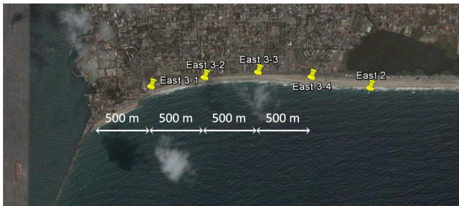
Figure 4-2: Locations of cross-shore profiles in the shadow zone of the East Mole [after Google (2010)]
