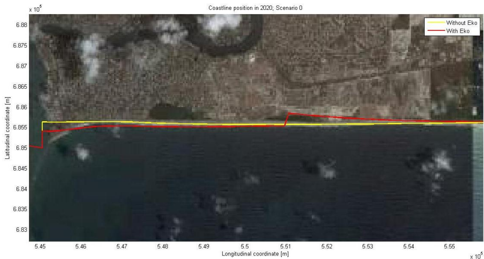
Figure 5-1: Coastline in 2020, for scenario 0. In yellow is the result of the model run without Eko Atlantic City, and in red with the land reclamation constructed
