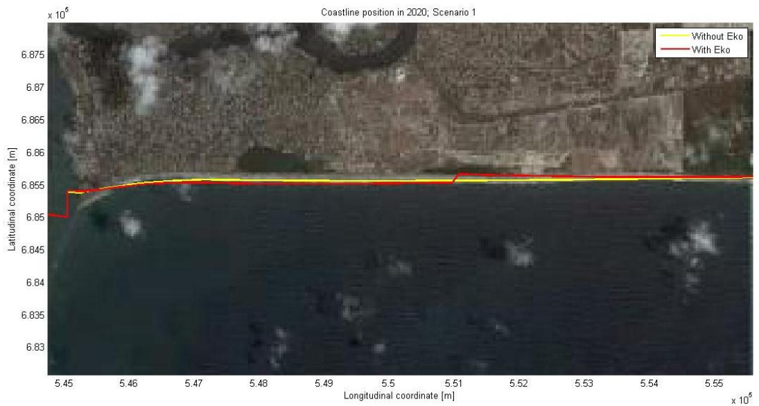
Figure 0-35: Coastline in 2020, for scenario 1. In yellow is the result of the model run without Eko Atlantic City, and in red with the land reclamation constructed
