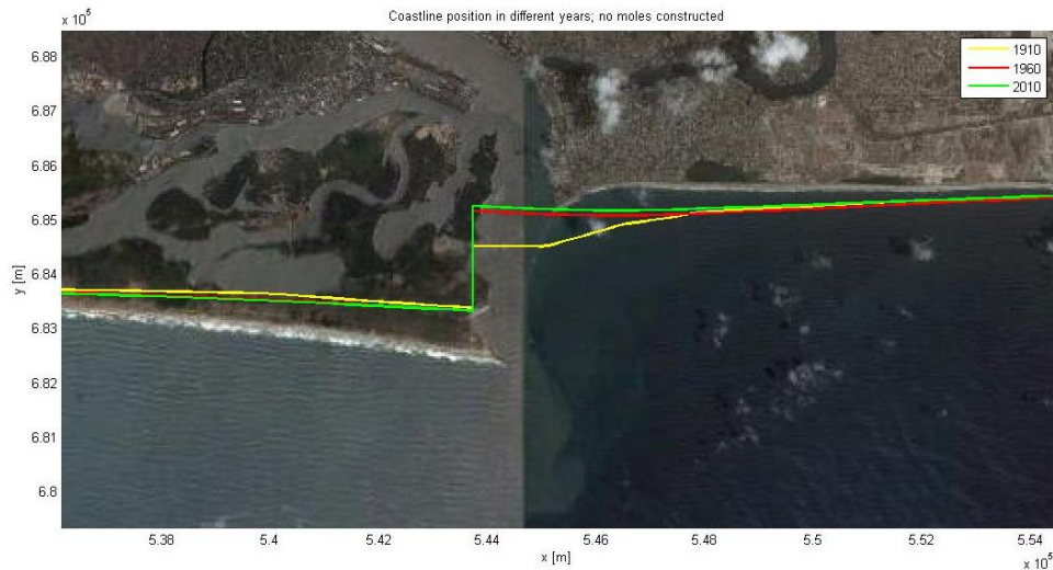
Figure 4-11: Coastline position in 1910 in yellow, 1960 in red and 2010 in green in scenario without Lagos Harbour Moles
