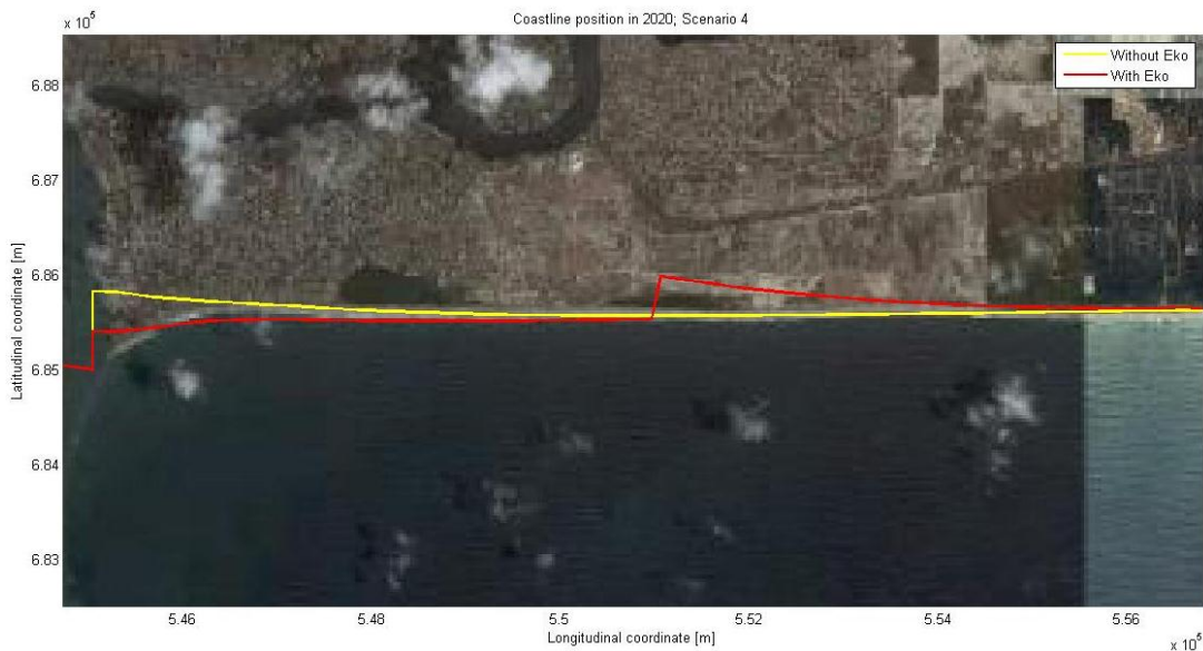
Figure 0-47: Coastline in 2020, for scenario 4. In yellow is the result of the model run without Eko Atlantic City, and in red with the land reclamation constructed
