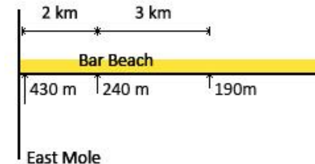
Figure 0-20: Sketch of erosion rates at Bar Beach, between 1960 and 2010, extracted from Figure 0-15
