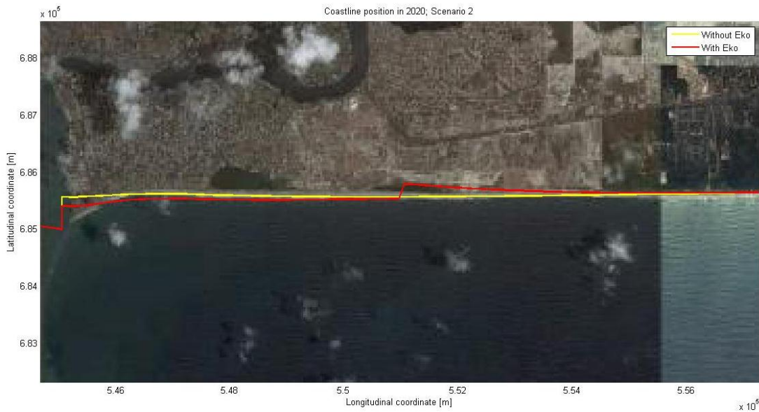
Figure 0-39: Coastline in 2020, for scenario 2. In yellow is the result of the model run without Eko Atlantic City, and in red with the land reclamation constructed
