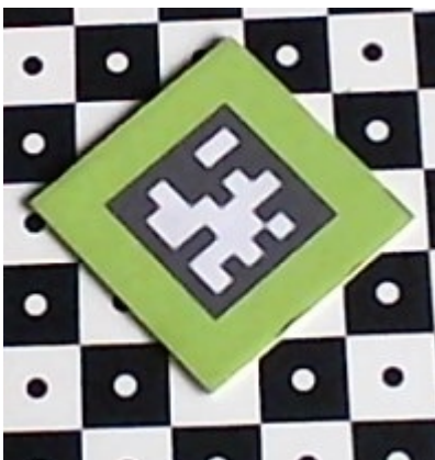
Figure 3.3: A marker that can be recognized by the Meta and the master camera.
