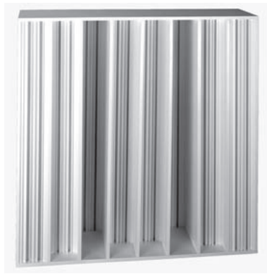
A DiffRACTAL®, which imbeds high frequency diffusers within a low frequency diffuser to deal with periodicity, absorption and bandwidth problems (top figure after D'Antonio and Konnert).
