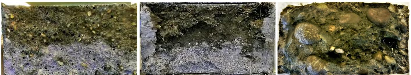
Figure 18: Chloride penetration uncracked samples: left – TC; middle – SSC; right – Concrete
