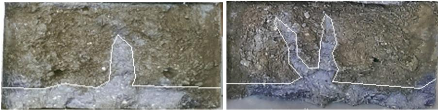
Figure 74: Chloride penetration cracked SSC samples
