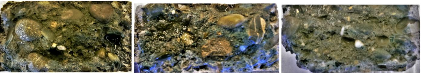
Figure 72: Chloride penetration uncracked Concrete samples
