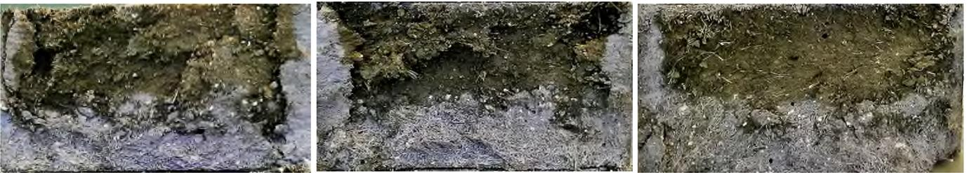
Figure 71: Chloride penetration uncracked SSC samples
