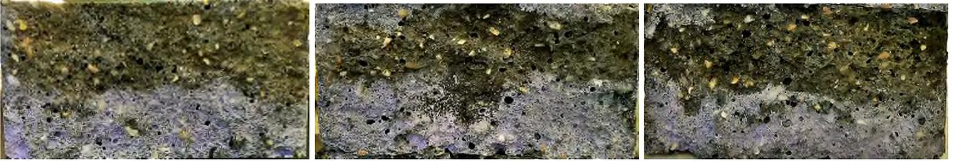
Figure 70: Chloride penetration uncracked TC mortar samples
