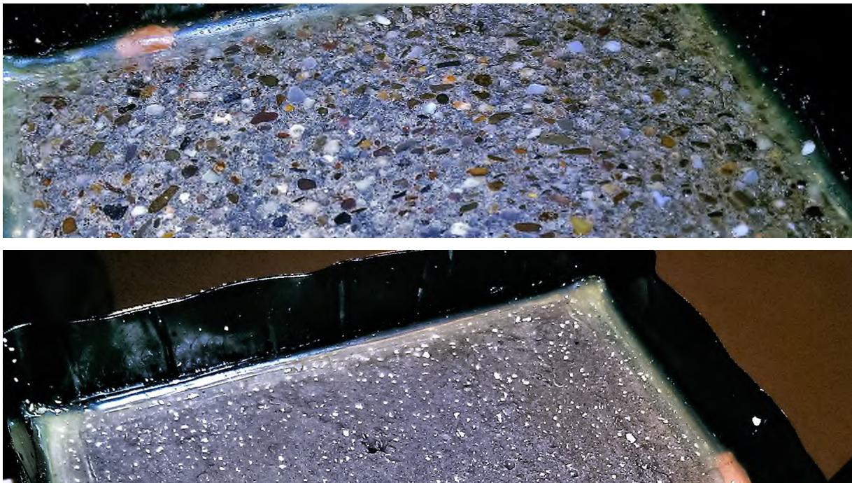
Figure 21: Surface after 21 frost/thaw cycles before healing period: top – TC mortar; bottom – SSC mortar
