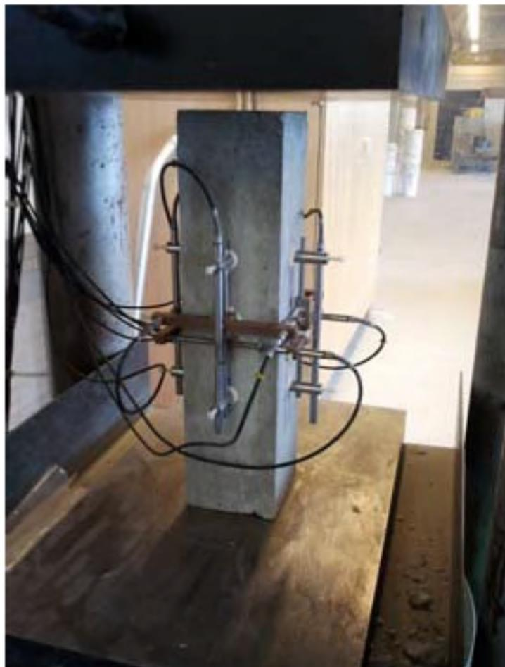
Increase the compressive strength with a constant speed (0,1 kN/s) until it equals 9 kN.
