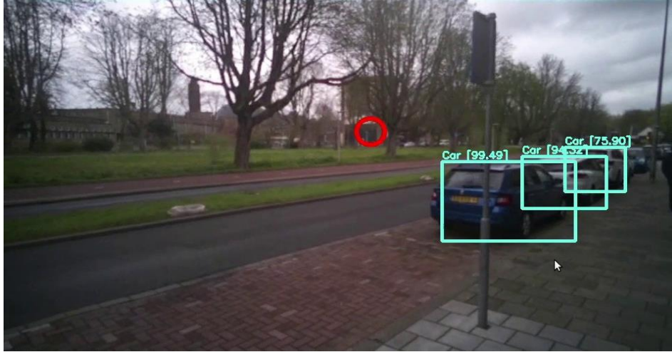
Figure 4. Object detection in a video frame. The object detection algorithm detects the vehicles in the frame and is highlighted by bounding boxes with the object class and confidence. The red marker signifies the gaze of the pedestrian in that frame.
