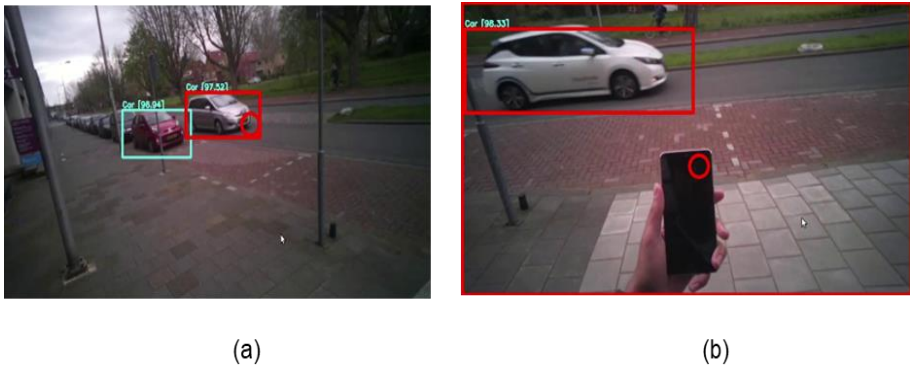
Figure 12. Moving car and mobile phone trials. Figure (a) illustrates the moving car trials where pedestrians look at the cars moving on the street. The red bounding box on the car shows that the car is moving. Figure(b) shows the mobile phone trials where the pedestrian constantly looks at his mobile phone. The red border on the image signifies an alert to the pedestrian about the approaching car.
