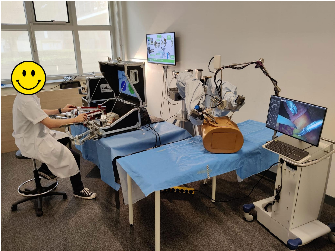
Fig. 1 The Sustainable ADLAP surgical robot platform that should foster the introduction of robotic surgery technology to less wealthy parts of the world
