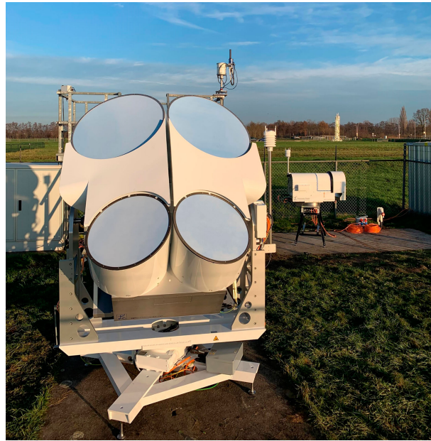
FIG. 4. Dual-frequency polarimetric scanning cloud radar (RPG-FMCW-DP-KW type), CLARA, after preliminary installation on the Cabauw site. The study case data were acquired in this configuration. Tiling and leveling the ground has been done afterward, including a 1-m platform for the radar. The radar is a frequency modulated continuous wave (FMCW) system with two antennas for transmission and reception at 35 and 94 GHz, top and bottom, respectively. On the right side, a pole carries the Vaisala meteorological weather station.
