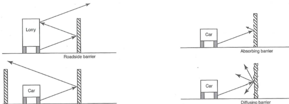
Fig.5.6 Schematic illustrating absorbers and diffusers to reduce reflection problems with noise barriers. (Cox, D'Antonio,2009, pg27)
