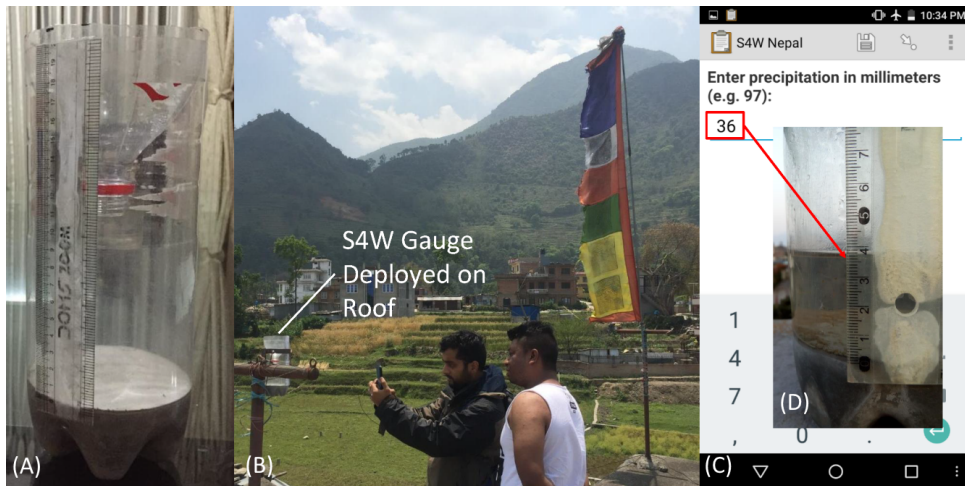
Figure 4.2: (A) Repurposed plastic bottle after placement of concrete, ruler, and inverted lid. (B) S4W gauge installed on the roof of a house in the Balkhu watershed (western Kathmandu Valley). The S4W-Nepal young researcher (dark jacket) is training the citizen scientist (white shirt) to take a precipitation measurement. After selecting the parameter to measure, the citizen scientist (C) entered their observation of precipitation (mm) and (D) took a picture of the water level in the S4W rain gauge before emptying it. Each record was reviewed by S4W-Nepal staff to ensure that the numeric entry from the citizen scientist (C) matches the photographic record of the observation (D). Any observed discrepancies were corrected, and records of edits were maintained.
