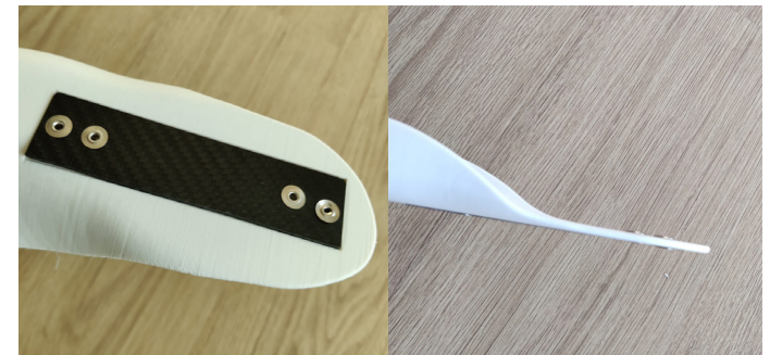
figure 79: An external ridged material such as a thin carbon plate can potentially be added to the SLS orthosis to create a more stiff footplate
