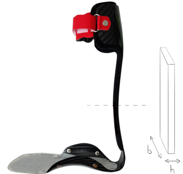
figure 35: Simplification of the carbon dorsal leaf spring strut as beam geometry
