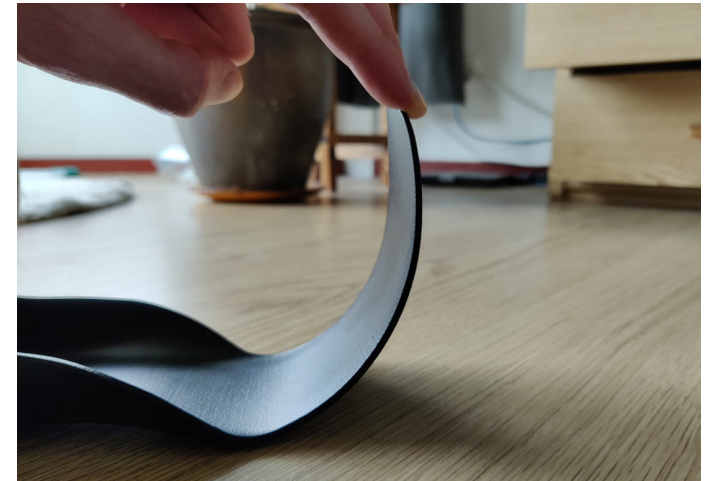
figure 78 The more flexible SLS printed footplate of prototype 2345644
