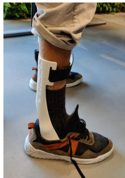
figure 34: FDM fitted orthosis with side struts. Proved too stiff to function
