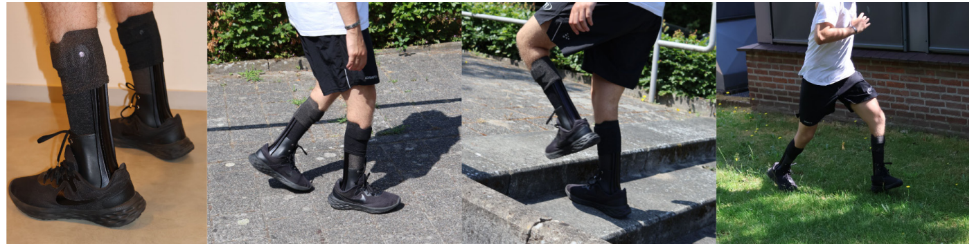
figure 87: The participant was asked to walk around, climb stairs and run whilst wearing the SLS AFO
