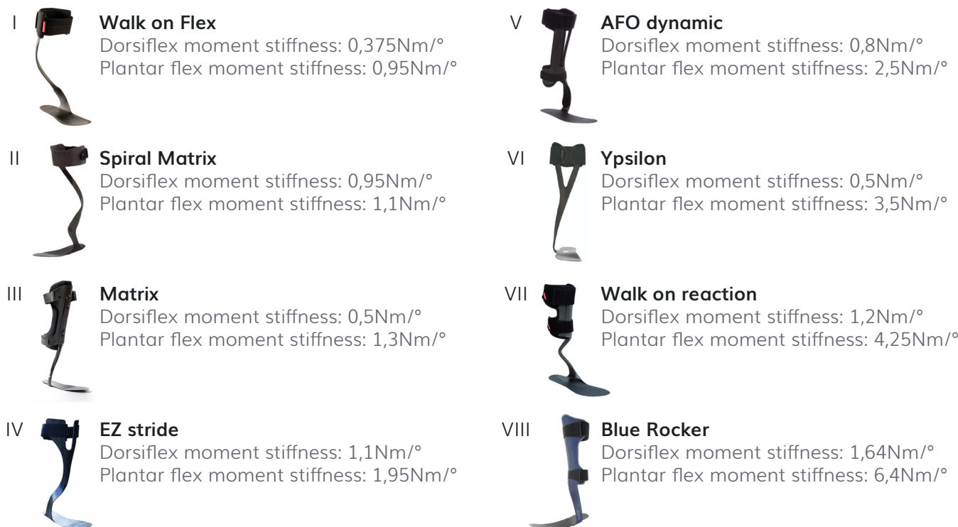
figure 21: Comparison graph of various PD-AFO's plantar flex and dorsiflex stiffness values
