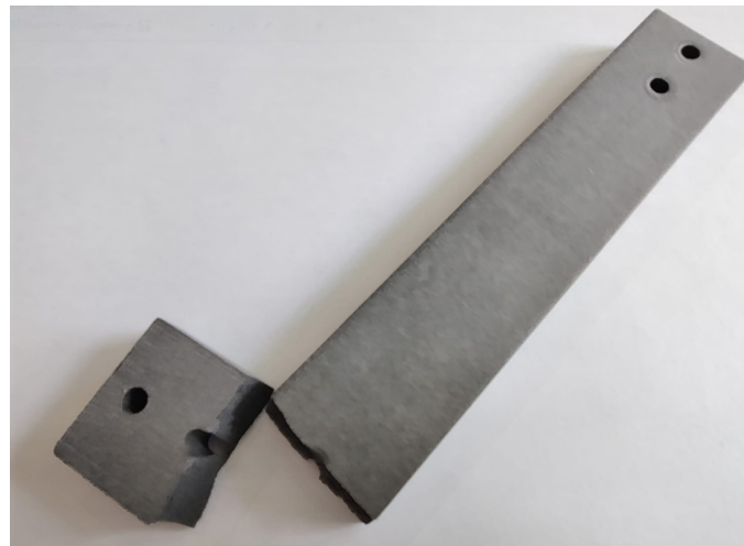
figure 38: breakline of carbonLW strut during measurements
