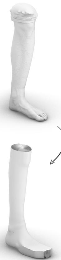
figure 81: From 3D scan, to cleaned up model
