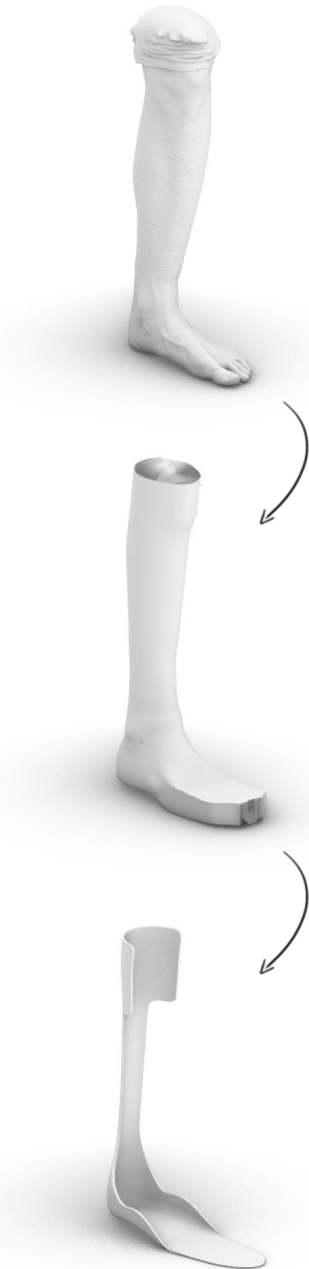
figure 82: From 3D scan, to SLS AFO
