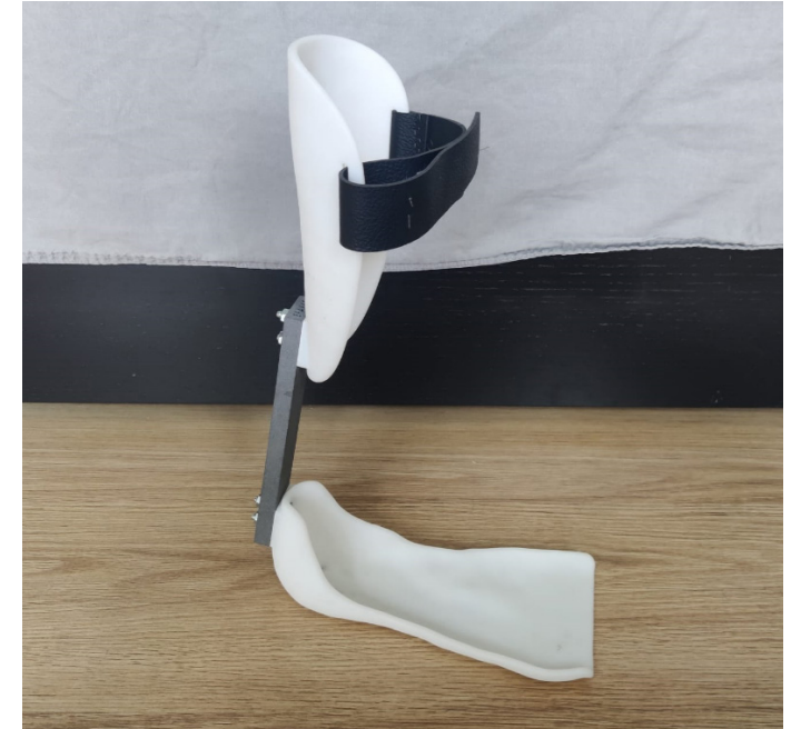
figure 37: 3 piece strut testing SLS printed model
