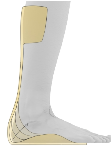
figure 48 Design opportunity; increasing AFO surface area around the heel increases stiffness
