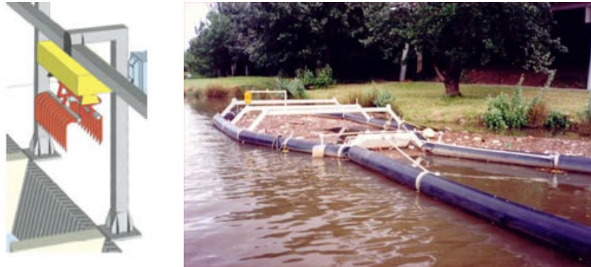
Figure B.9 Impression of raking machine 24 and a floating litter trap 25
