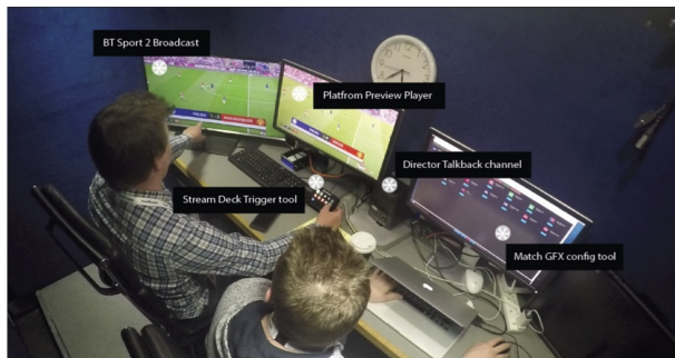
Figure 8: The setup of the system in the OB truck at the stadium
