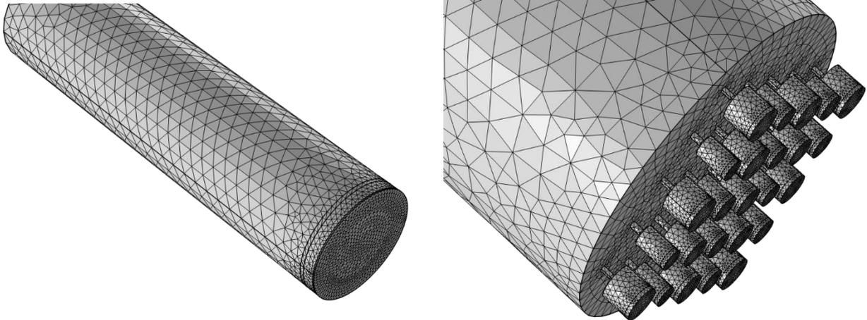
**Figure 7.2:** The used model mesh. A fine mesh was used both for the smaller geometries but also for the area representing the impedance tube interior.
