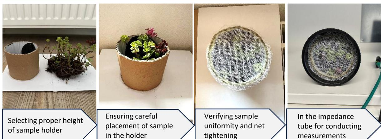
**Figure 5.8:** Procedure of preparing the vegetation blanket samples to fit in the impedance tube.
