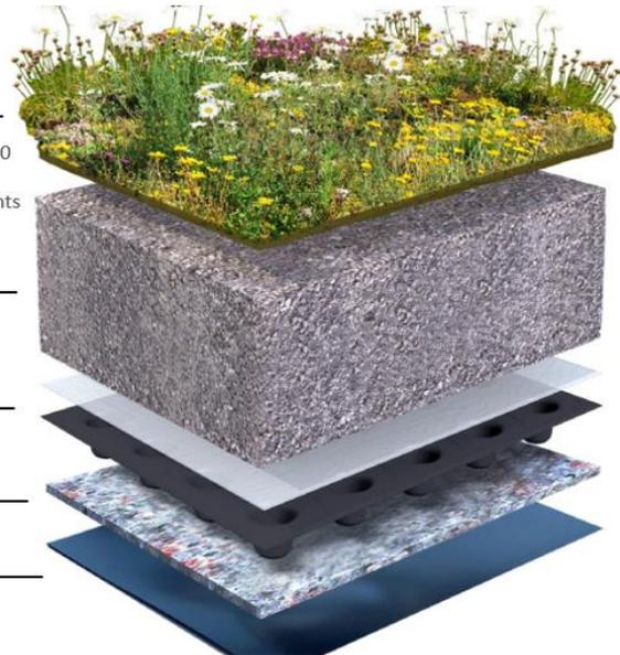
**Figure 5.4:** Cross section of the Sempergreen Biodiverse Green Roof (retrieved online from Sempergreen).
