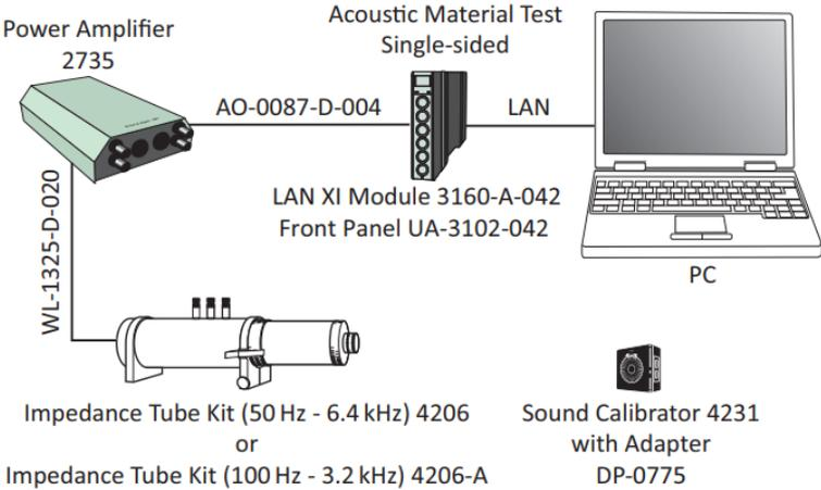
**Figure 5.10:** Schematic illustration of the measurement set up kit from Brüel & Kjær.
