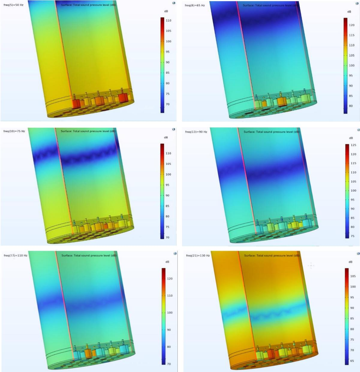
**Figure 7.11:** Total sound pressure level distribution at various frequencies (50, 65, 75, 90, 110 and 130 Hz) in the green roof-resonators system (Results extracted from concept E).
