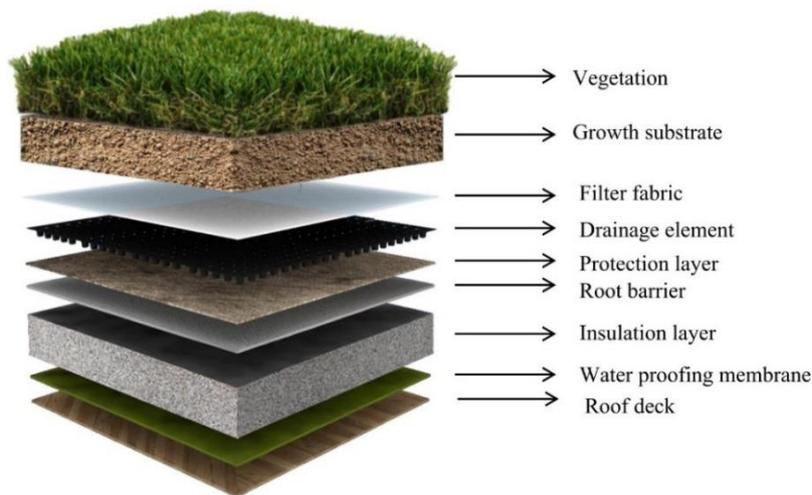
**Figure 2.1:** Schematic cross section of a typical green roof structure layering (retrieved from Vijayaraghavan, 2016)
