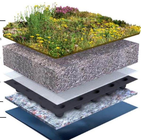
**Figure 5.5:** Cross section of the Sempergreen Lightweight Biodiverse Roof (retrieved online from Sempergreen)
