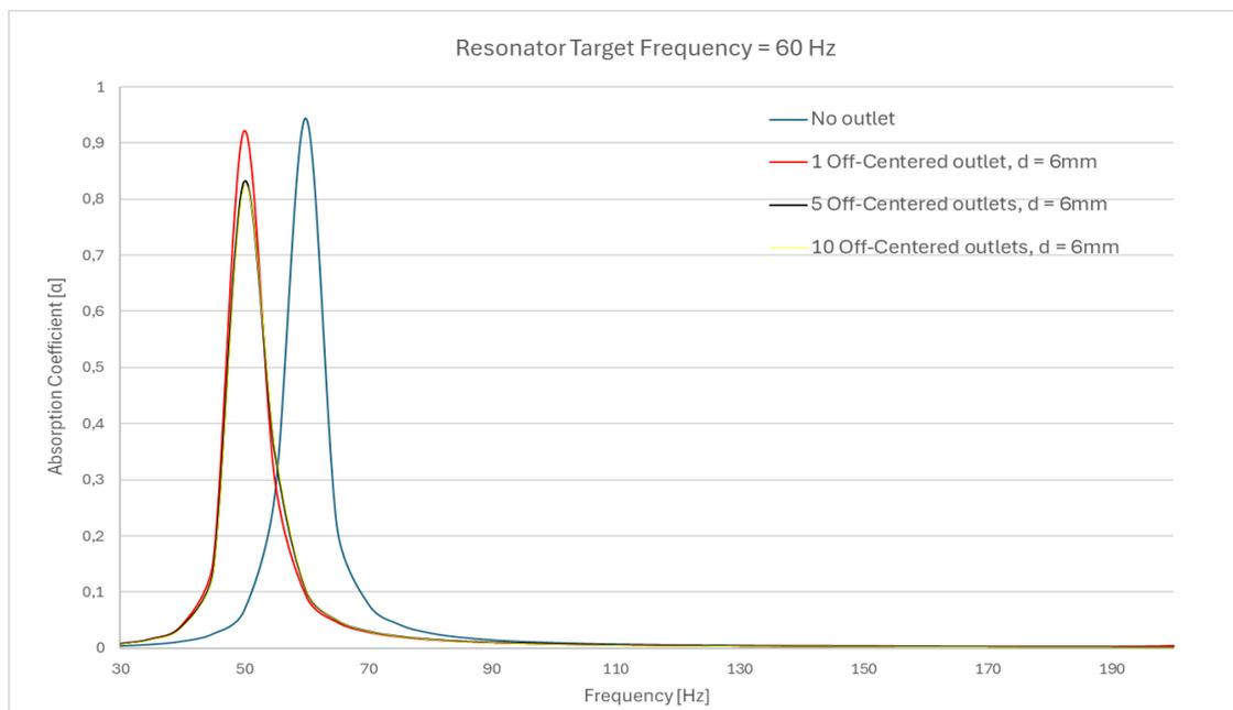
**Figure 7.7:** The influence of perforations' number on the maximum absorption coefficient value.
