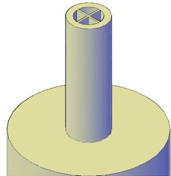
**Figure 7.13:** Introduction of cross-structure fins inside the resonator's neck.
