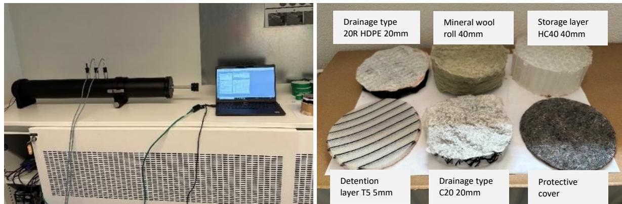
**Figure 5.7:** Left: The Impedance Tube setup used for measurements. Right: The different materials needed for the examined systems adjusted in circular shape with a diameter of 10 cm.
