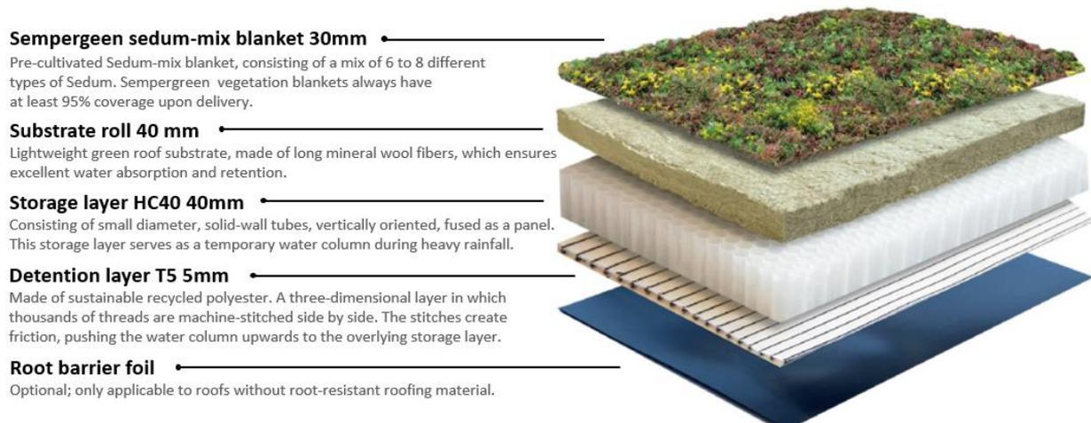
**Figure 5.6:** Cross section of the Sempergreen Detention Roof (retrieved online from Sempergreen).
