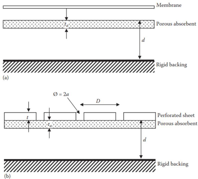
**Figure 4.2:** Schematic illustration of a typical construction of: (a) panel/membrane and (b) Helmholtz absorbers (retrieved by Cox and D’Antonio, 2016).
