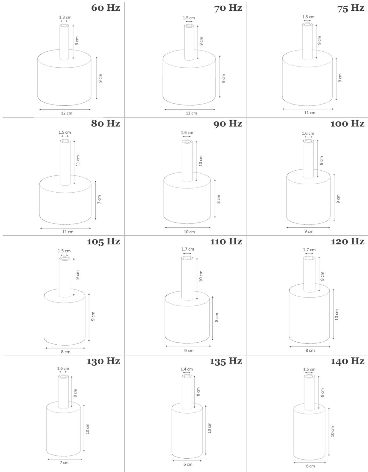
**Figure 7.4:** An overview of the resonator configurations used for the acoustic analysis.
