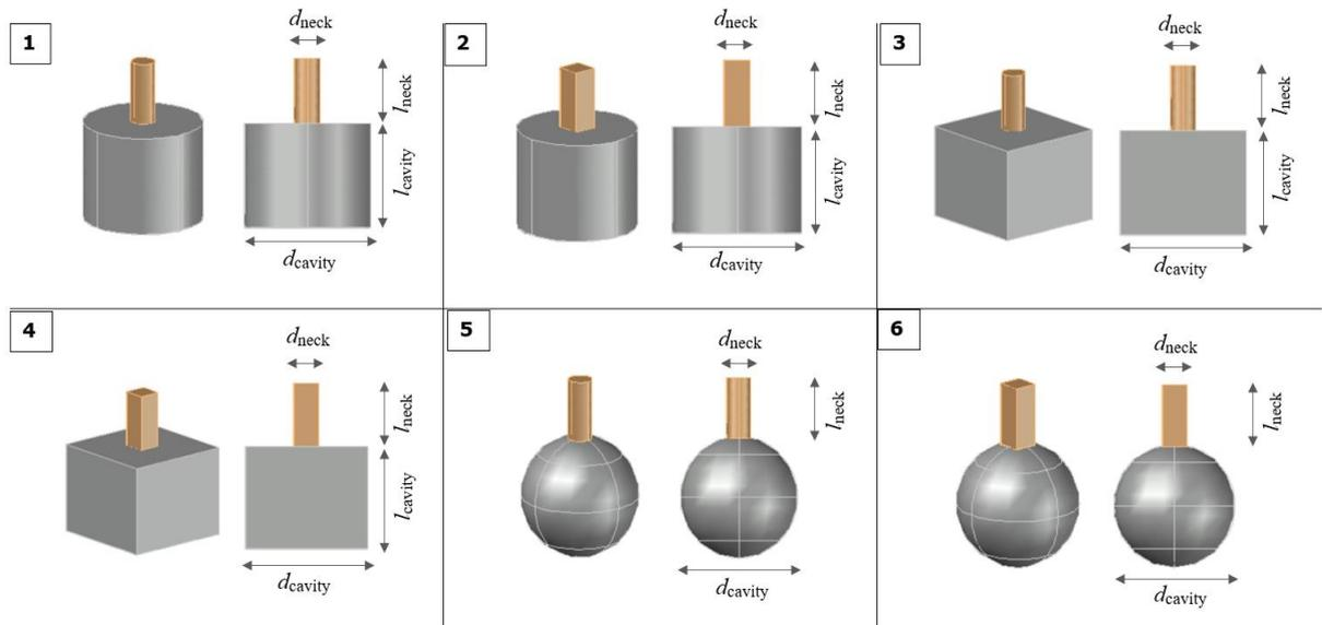
**Figure 6.3:** Different resonators configurations. Three different cavity shapes in combination with two different neck shapes.
