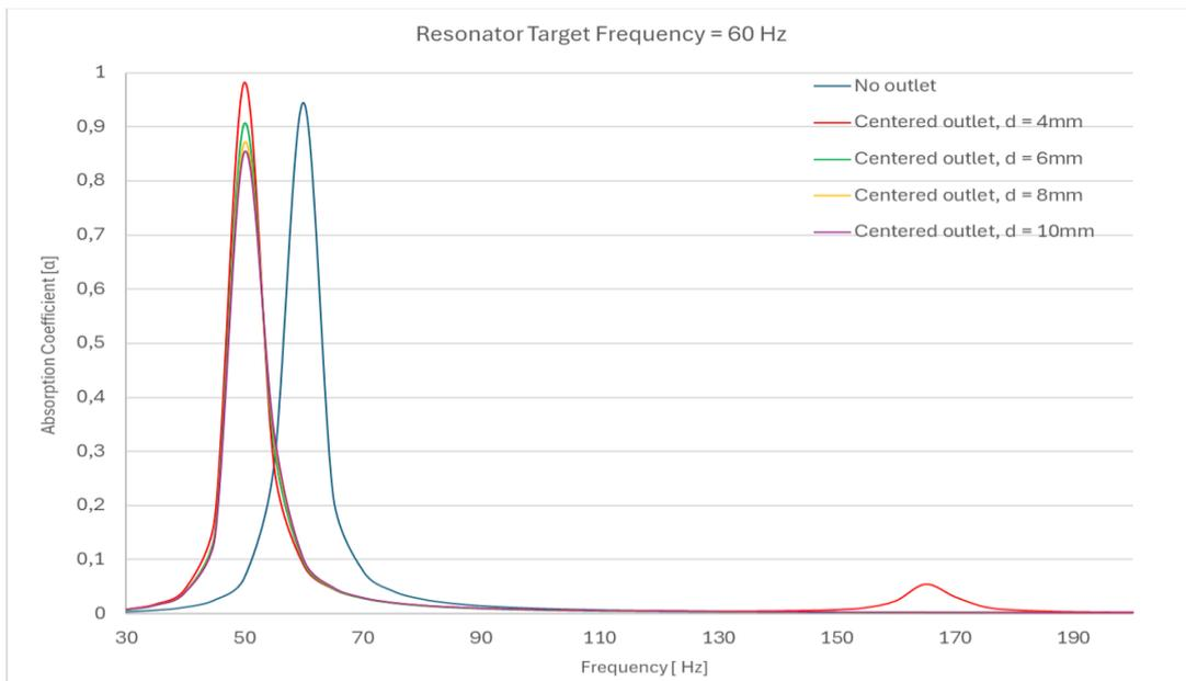
**Figure 7.5:** The effect of the outlet perforation's size on the resonator's frequency peak (case: centered perforation).
