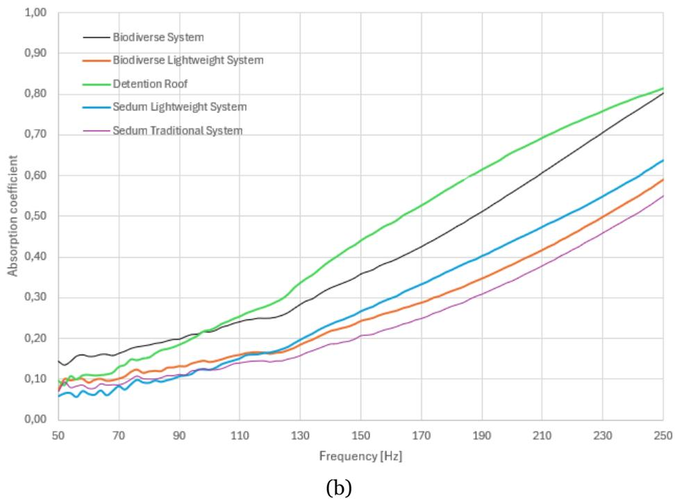
**Figure 5.11:** Graphic representation showing the sound absorption coefficient of the five green roof systems tested as a function of frequency for : (a) overall frequency performance (50 Hz – 1600 Hz) and (b): low-frequency performance (50 Hz – 250 Hz)
