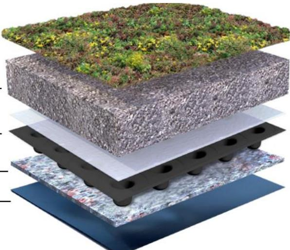
**Figure 5.2:** Cross section of the Sempergreen Traditional Sedum Roof (retrieved online from Sempergreen).
