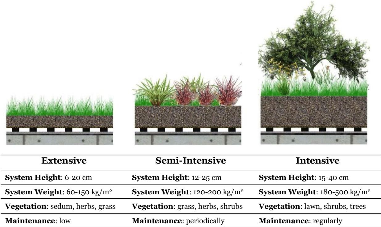
**Figure 2.2:** Classification of green roof systems according to construction factors, vegetation type and maintenance requirements. (Configurations and technical characteristics retrieved from Raji *et al.*, 2015)
