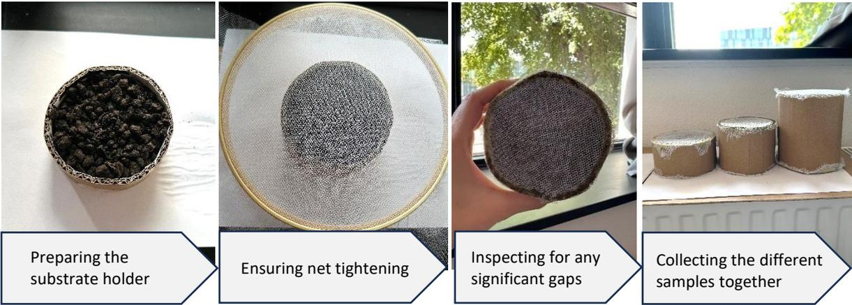
**Figure 5.9:** Procedure of preparing the extensive substrate test samples to fit in the impedance tube.
