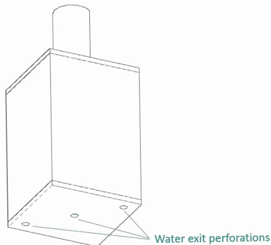
**Figure 6.2:** Schematic representation of the small exit perforation concept at the cavity base of the resonator.
