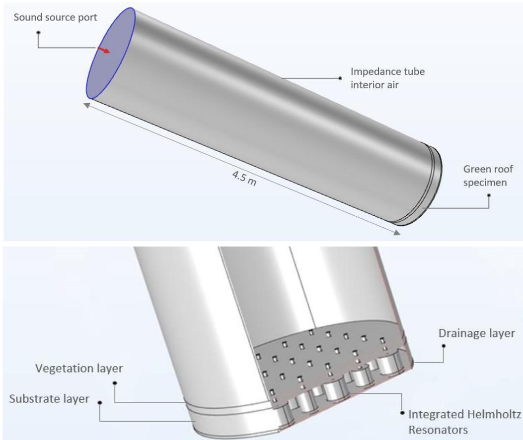
**Figure 7.1:** Geometry-Impedance tube model setup used in COMSOL.
