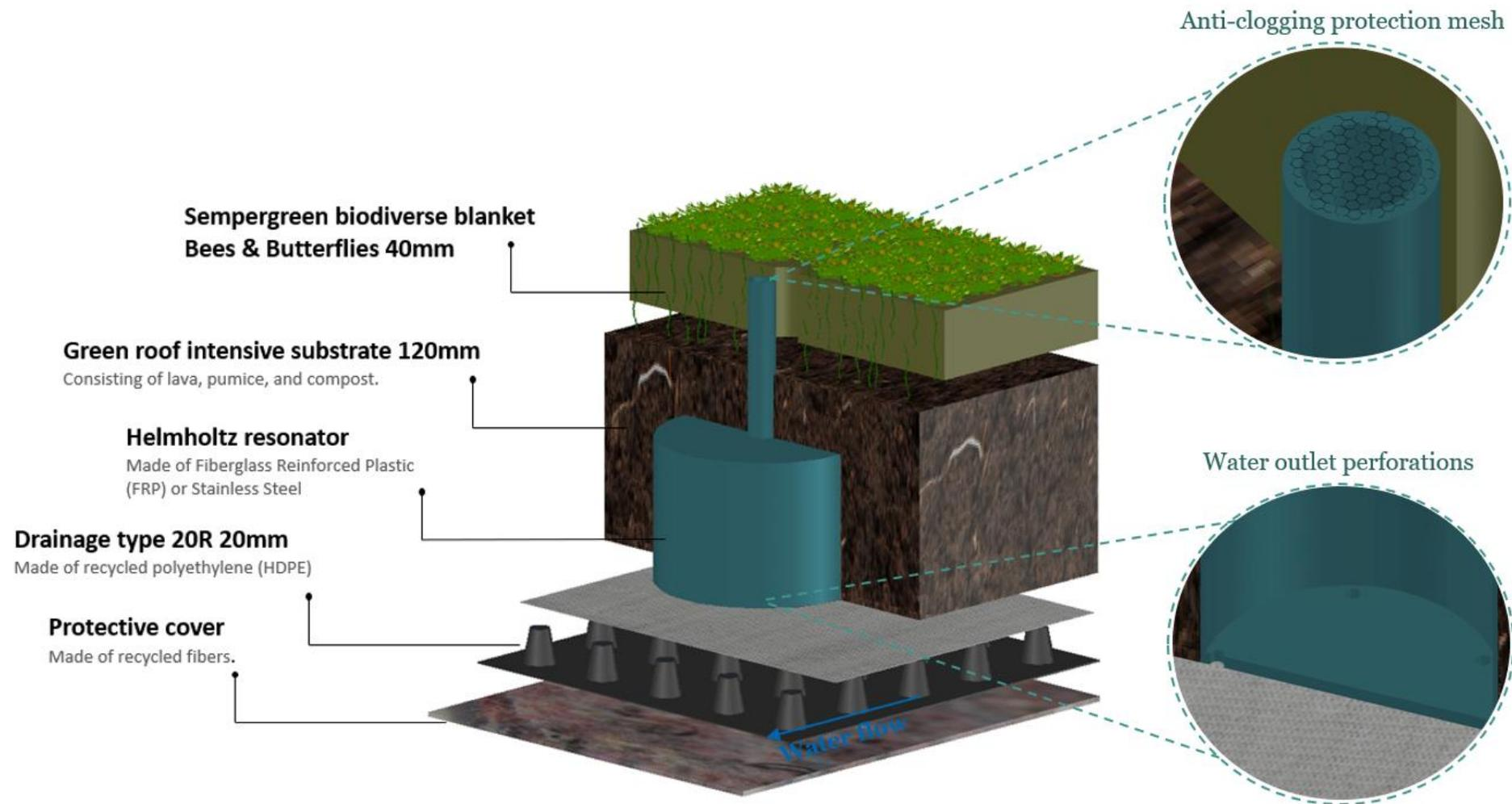
**Figure 6.5:** Key design features of the concept desi
