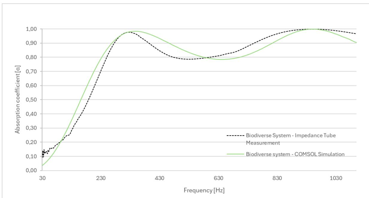
**Figure 7.9:** Graphic representation of the sound absorption coefficient as a function of frequency for the biodiverse system as occurred from the impedance tube measurement (black-colored line) and the simulation (green-colored line).
