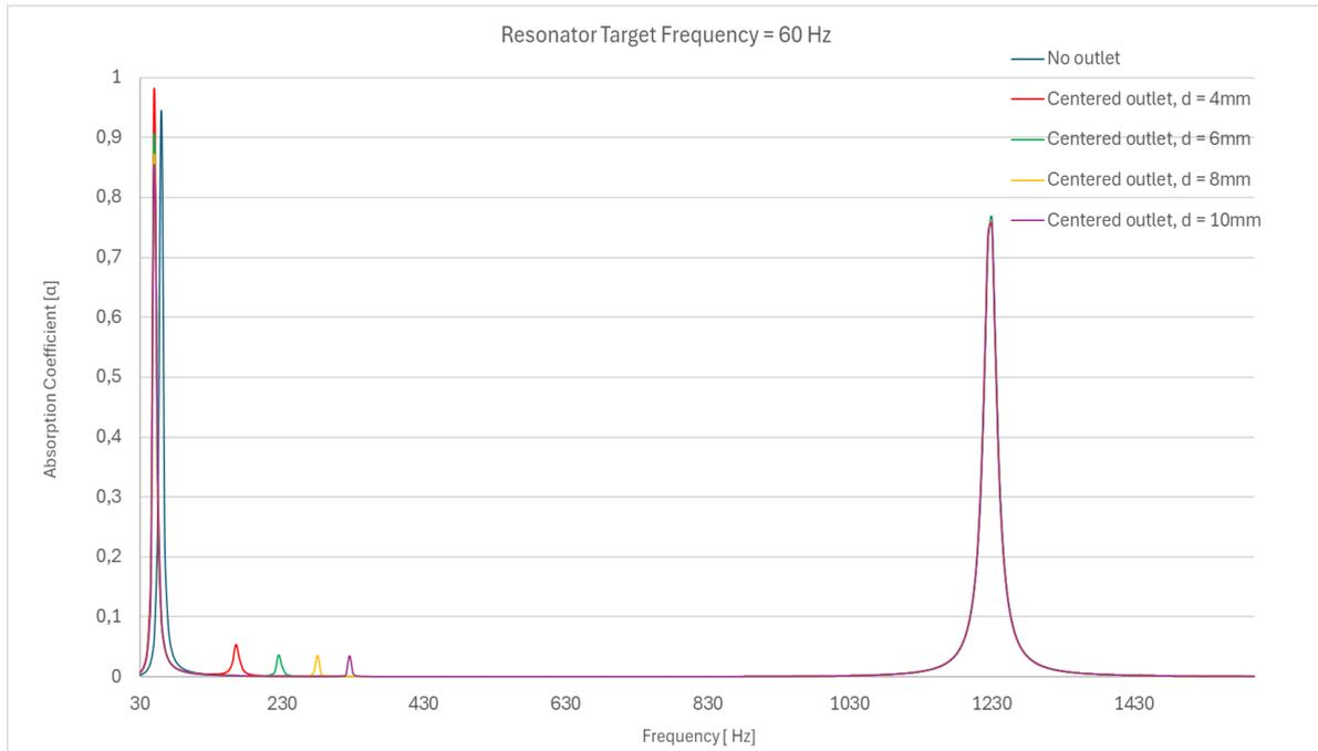
**Figure 7.8:** The introduction of secondary absorption peaks at higher frequencies.
