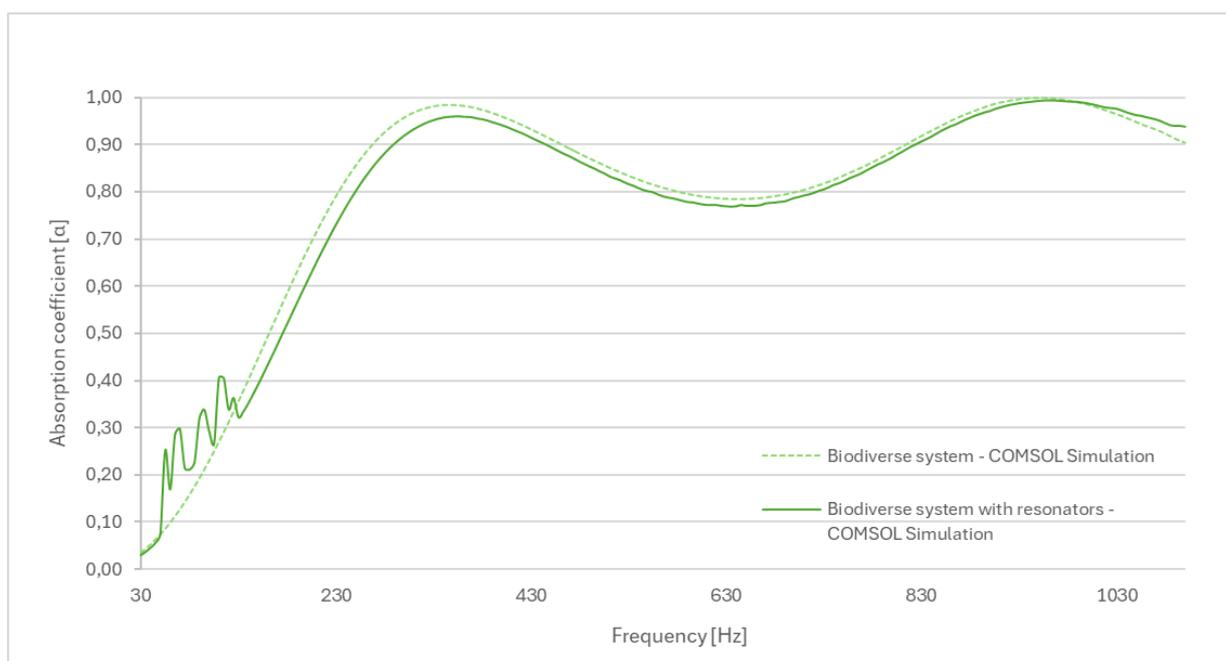
**Figure 7.10:** The influence of adding resonators on the Biodiverse system's acoustic performance.
