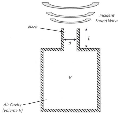
**Figure 4.3:** Cross section of a typical cavity Helmholtz resonator (reproduced from Godbold, 2008).
