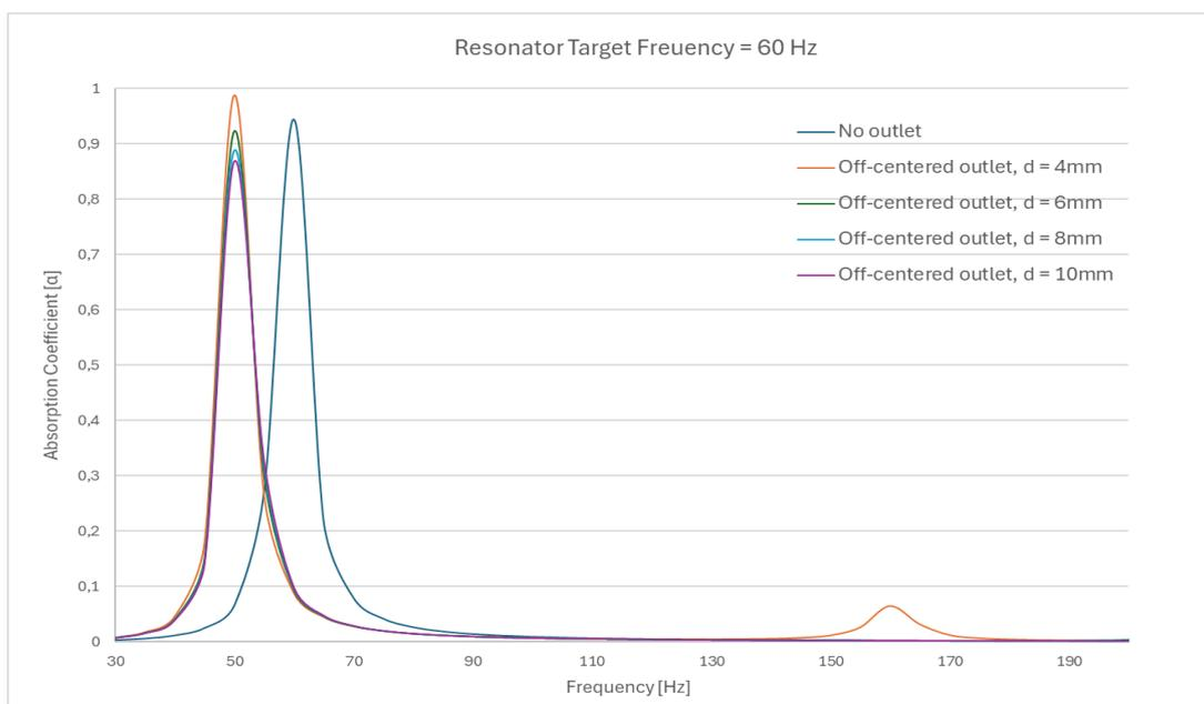
**Figure 7.6:** The effect of the outlet perforation's size on the resonator's frequency peak (case: off-centered perforation)
