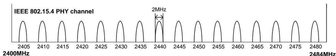
**Figure 2.1 ZigBee channels in 2.4GHz band**
