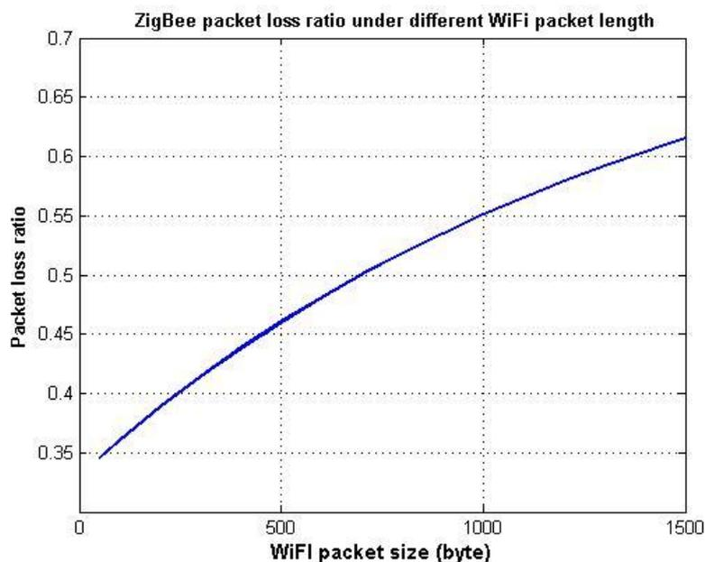
Figure 4.4 ZigBee packet loss ratio under saturated WiFi traffic (from [4])
