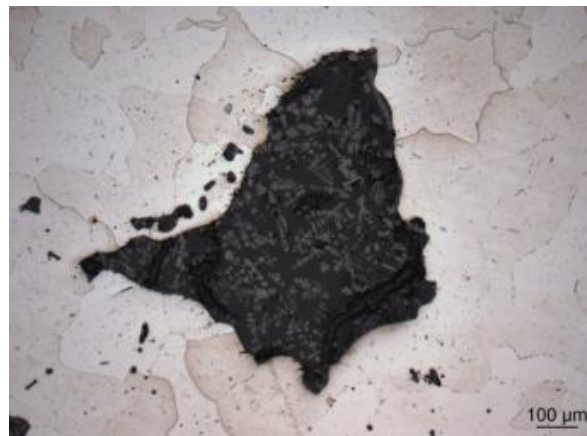
Figure 2.10: slag inclusion under an optical microscope [10].
