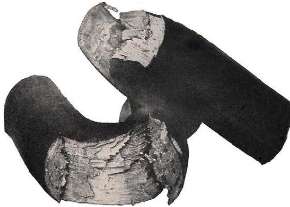
Figure 2.5: Fibrous nature of wrought iron [9].
