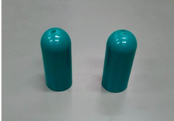
**Figure 3.7:** EP-I coated small size electrodes.
