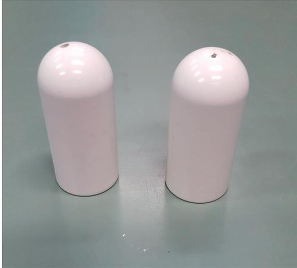
**Figure 3.12:** PA11 coated small size electrodes.
