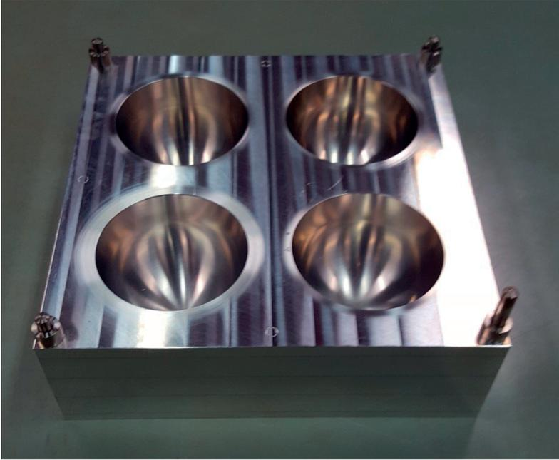
**Figure 3.21:** Mould for large size electrodes, bottom part.
