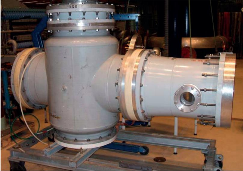
Figure 3.1: Picture of test setup GIS enclosure
