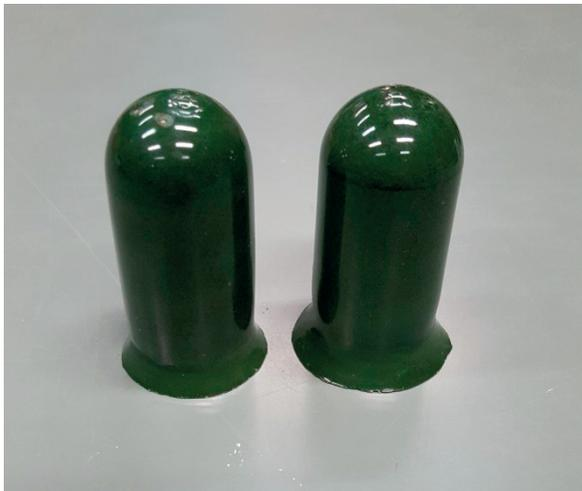
**Figure 3.13:** Semiconductor A coated small size electrodes.
