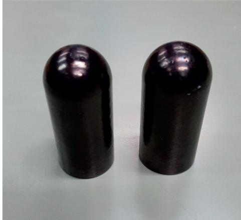
**Figure 3.9:** FP-II coated small size electrodes.
