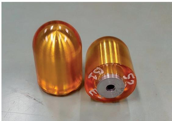
**Figure 3.16:** Neat epoxy coated small size electrodes.
