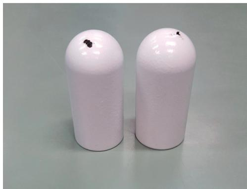
**Figure 3.15:** FP-II + PA11 coated small size electrodes.
