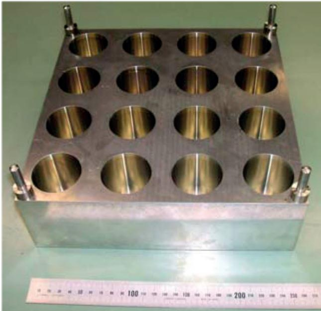
**Figure 3.19:** Mould for small size electrodes, bottom part.
