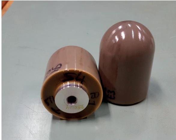
**Figure 3.17:** Nanocomposite B coated small size electrodes.
