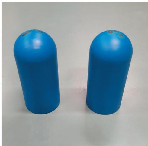
**Figure 3.10:** FP-III coated small size electrodes.
