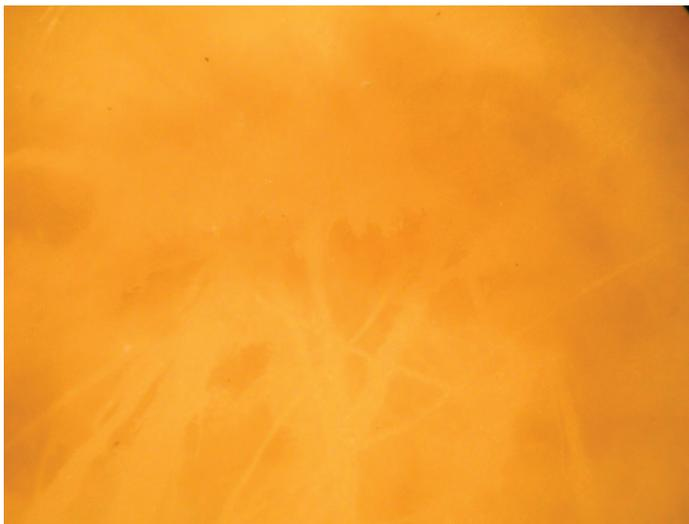
**Figure 5.45:** Microscopic view of the surface of a thick nanocomposite coated electrode after a breakdown test.
