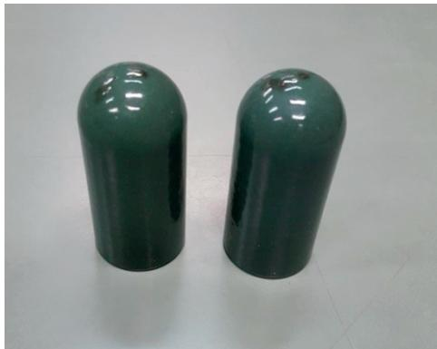
**Figure 3.8:** FP-I coated small size electrodes
