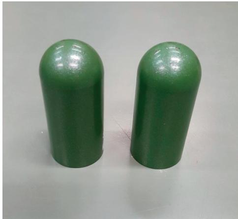
**Figure 3.11:** FP-IV coated small size electrodes.
