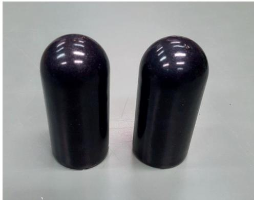
**Figure 3.14:** FP-II + FP-I coated small size electrodes.
