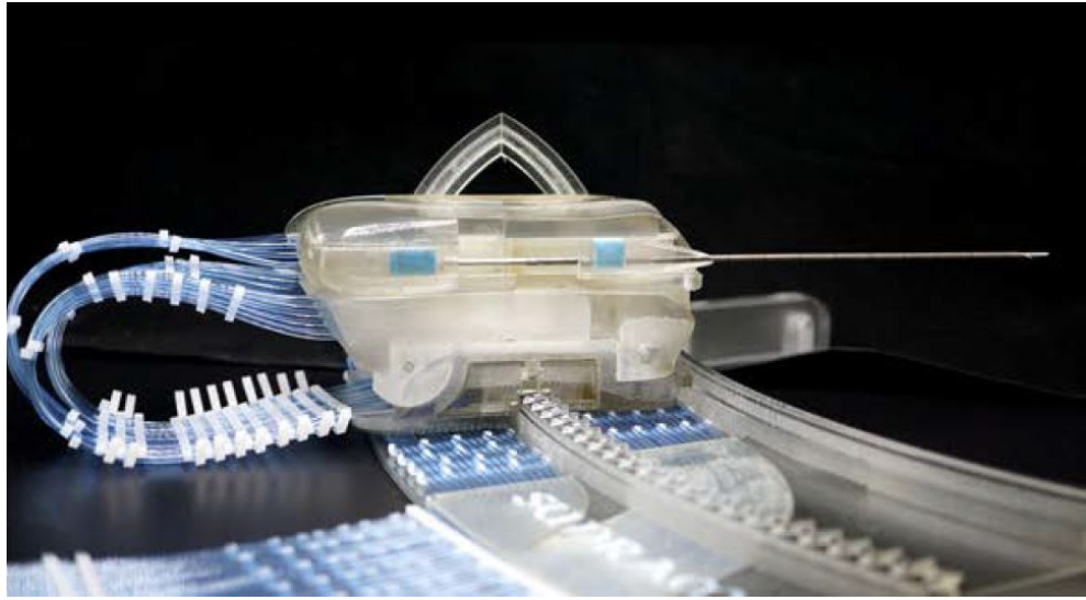
Figure 1.1: Sunram 5, a needle positioning robot with pneumatic stepper actuation by [Groenhuis et al., 2020]
