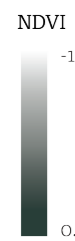
Figure 5.5 The NDVI is a graphical indicator of the amount and type of vegetation in an area. Values in between -1 and 0 usually correspond to areas with rocks or covered with pavement. Values in between 0 and 0.6 usually indicate the presence of low vegetation and values closer to 1, usually indicate the presence of high and dense vegetation. With the help of surface analysis tools in ArcGIS PRO, this index was created in order to show which areas have more or less soil permeability according to if they are paved or not. (Elaborated with data from USGS, 2019)
