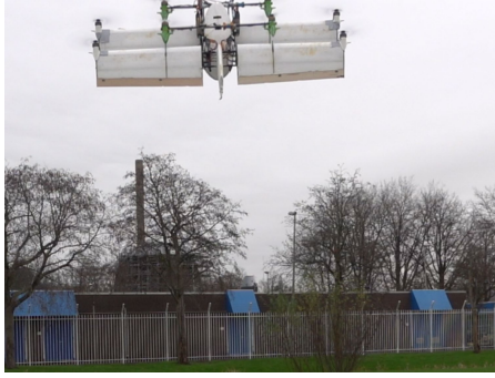
(b) Release mechanism is engaged; The quadrotor has no attitude control.
