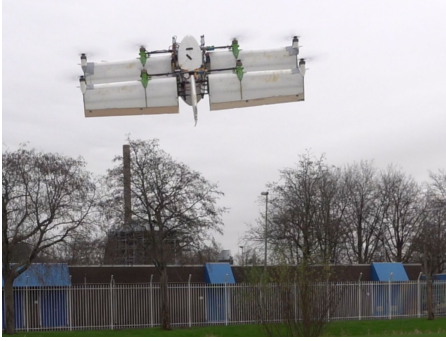
(a) Joint hover; Biplane in attitude INDI and quadrotor constant 70% thrust.
