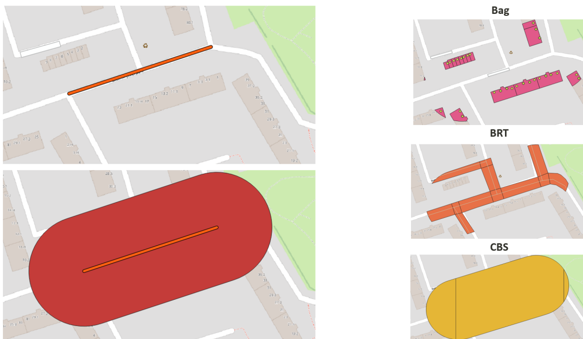
Figure 4.9: Example of clipping GIS databases with buffer around project trace
