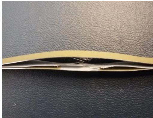
Figure 6: Typical behaviour of the tensile samples (GLARE3-2/1 in L-direction)
