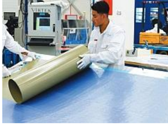
Figure 2: Layup process for panels made from GLARE
