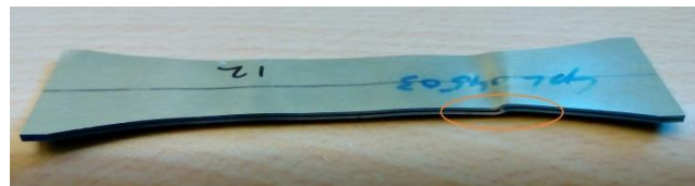
Figure 9: Typical behaviour of the samples with gaps during compression tests (L-dir gap, Al th.=0.3mm)
