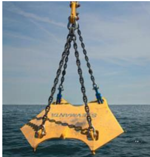
Figure 2.8: Vertically Loaded Anchor Stevmanta (VRYHOF 2018).
