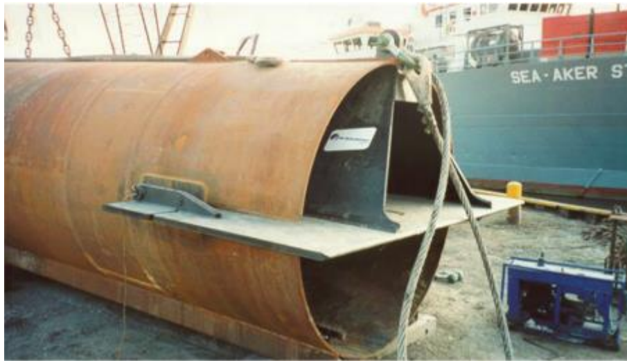
Figure 2.10: A plate anchor positioned at the tip of the follower (Chao and Eng 2016).
