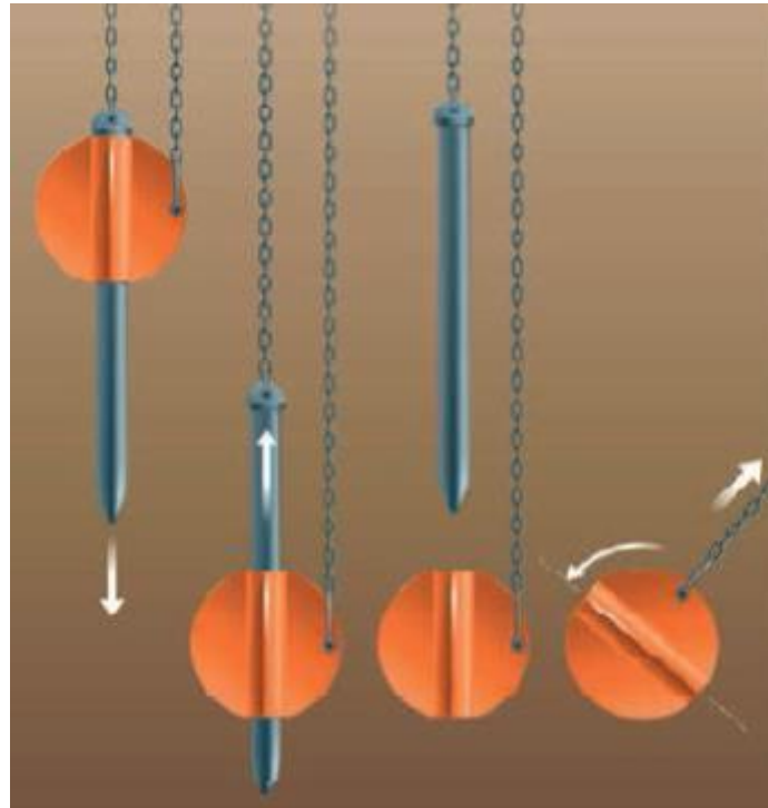
Figure 2.11: Installation and keying of a DEPLA (Da Silva 2021).
