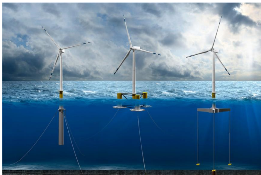
Figure 2.1: Floating wind turbine structures. From Left to Right: Spar, Semi-submersible, and TLP (Barter et al. 2020).
