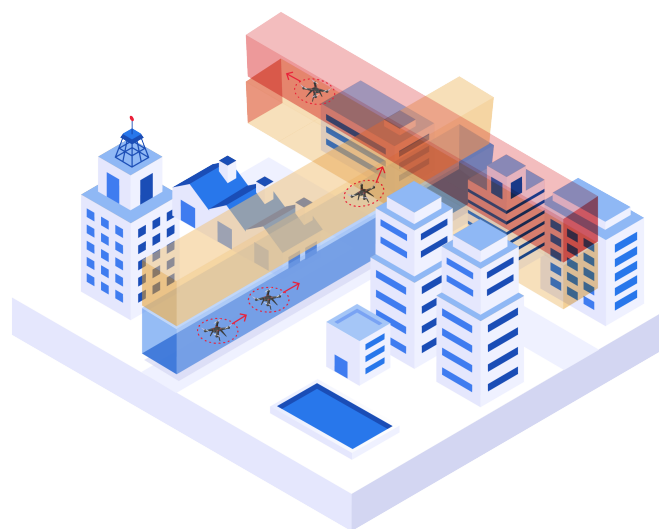
Figure 2. Constrained airspace intersection example. Note how the blue and red cruise layers are vertically separated and contain a turn (yellow) layer in between. Note that this pattern is stacked until the top of airspace. The red circles and arrows signify the protected zone and current direction of travel of the drones, respectively.
