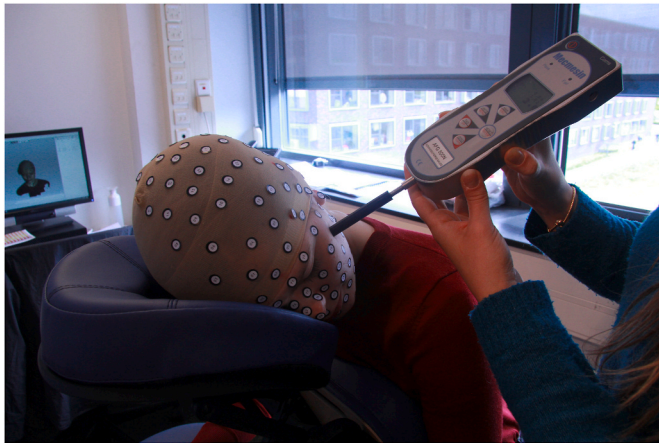
Fig. 1. Mecmesin AFG 500N pressure gauge with 3D printed PLA Ø10 mm tip, and participant with EEG 10–20 landmark grid headcap and landmark stickers on the face, head and neck. Researcher gradually increasing pressure on a landmark with pressure gauge until the participant indicates the PDT has been reached.
