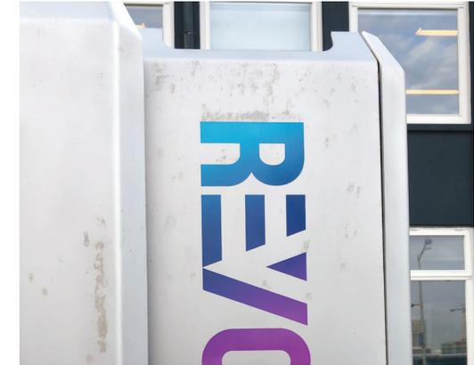
Figure 37. Rust on stainless steel surface
