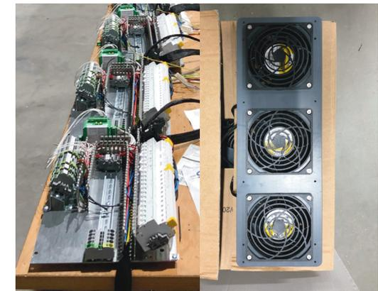
Figure 35. Pre-manufactured ventilation grid and AC charging components
