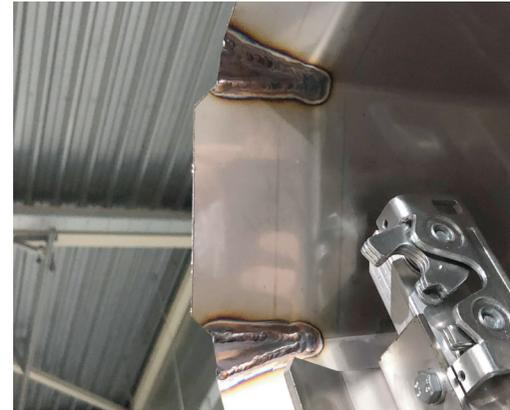
Figure 36. Stainless steel welding
