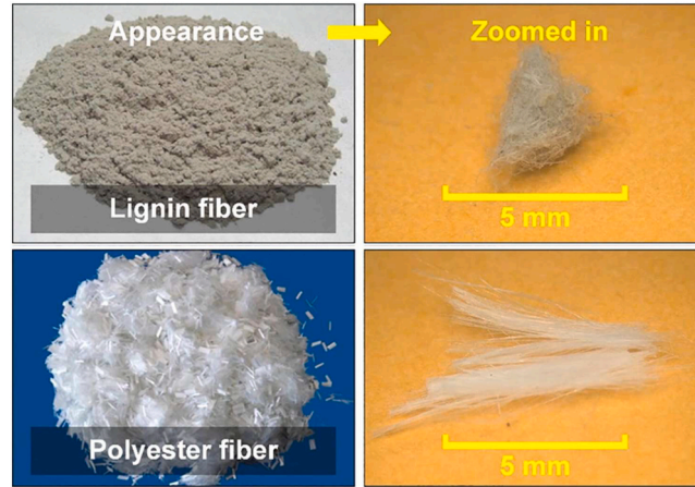
Fig. 2. View of lignin fiber and polyester fiber.
