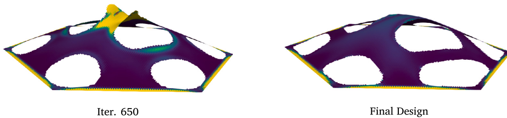
Fig. C.16. 3D rendering of the linear modal stiffnesses depicted in Fig. 10, for iteration 650 and the final design. A threshold of \bar{\rho}_I^e \geq 0.5 and a domain deformation corresponding to the fundamental mode shape was applied for clarity.
