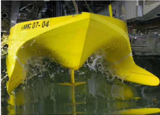
Fig. 5. 2.5 m hydroelastic catamaran model based on the 112 m wave-piercer catamaran shown tested in irregular head-seas with ride control using active stern tabs and centrally mounted T-foil (Javanmard et al. 2023).
