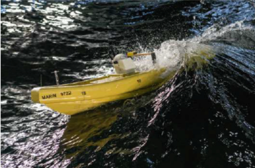
Fig. 1. Model of landing vessel shipping water, after van Walree and Thomas (2023)
