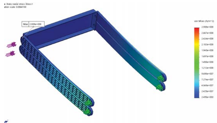
▲ Figure 76: Von Mises stress (N/m 2 ) due to a side-to-side force of 200N. Showing a maximum stress of 2.9 \cdot 10^8 (N/m 2 ) for diagonals made out of ABS. The maximum stress exceeds the yield strength of around 3 to 6 \cdot 10^7 (N/m 2 ): the construction deforms plastically.
