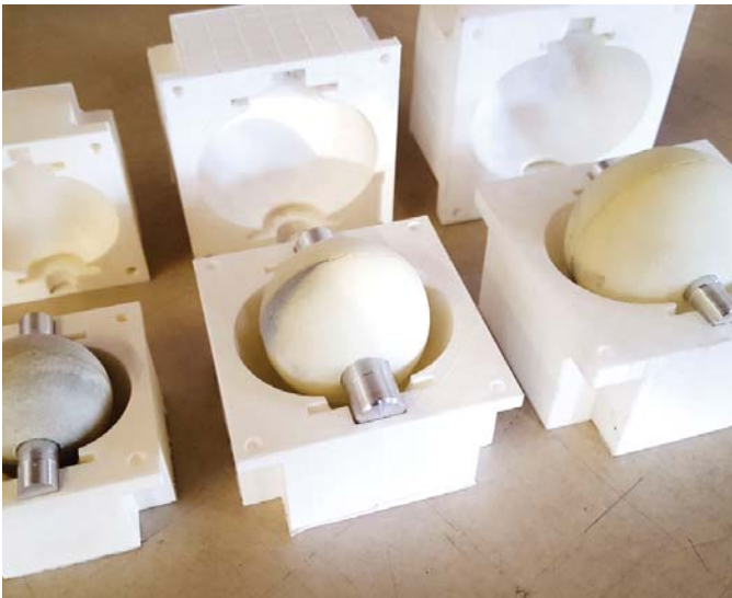
▲ Figure 45: small, medium and large rubber damping balls were poured with self-made molds.
