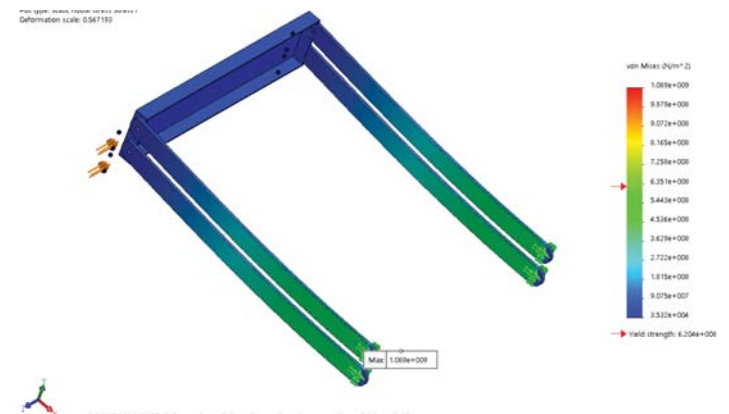
▲ Figure 73: Von Mises stress (N/m 2 ) due to a side-to-side force of 200N. Showing a maximum stress of 1.089 \cdot 10^9 (N/m 2 ) for a steel construction. The maximum stress exceeds the yield strength of 6.2 \cdot 10^8 (N/m 2 ): the construction deforms plastically.
