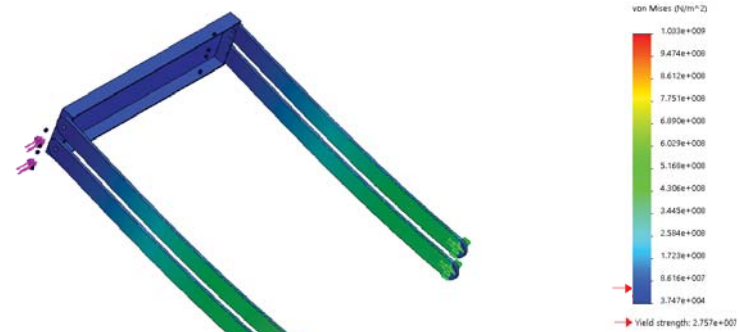
▲ Figure 69: First iteration of the new double diagonal construction. Showing a 4 mm thick plate
