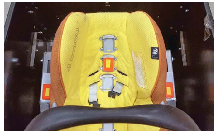
▲ Figure 99: Transducers were placed on each side of the mechanism (steel prototype)
