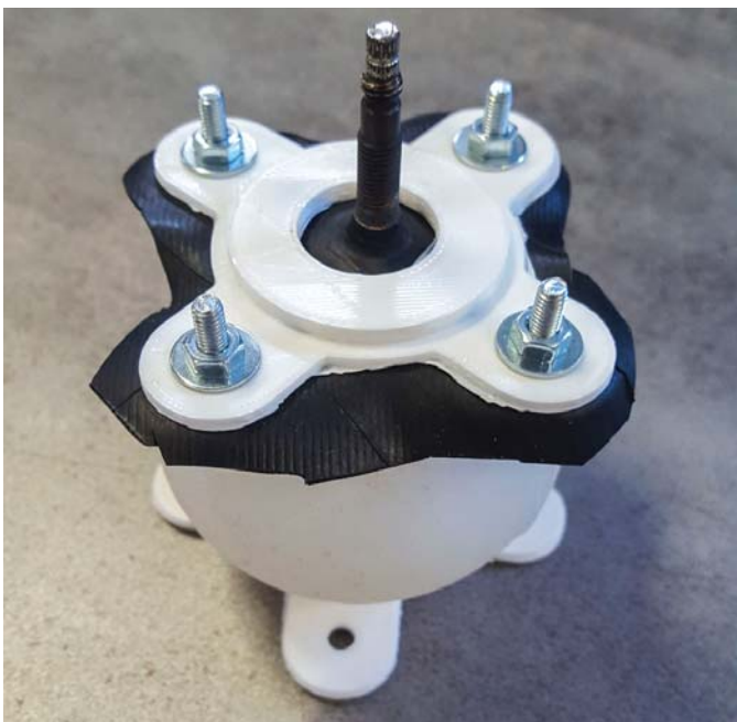
▲ Figure 48: Possibilities were being evaluated to make rubber damping balls airtight. This would create some sort of air suspension.
