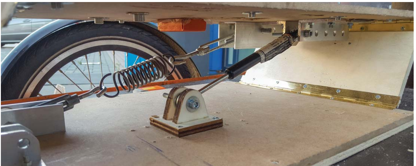
▲ Figure 55: A gas spring pushes with a constant and preset force. Whether the system worked, depended on the resulting force between the gas spring, the tension spring and the weight that was laid on the parallelogram.
