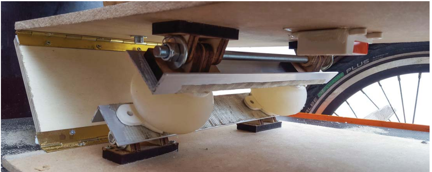
▲ Figure 54: Placing one rubber damping ball was insufficient to withstand the weight that was placed on the parallelogram: the rubber damping ball collapsed. Placing two rubber damping balls worked better.
