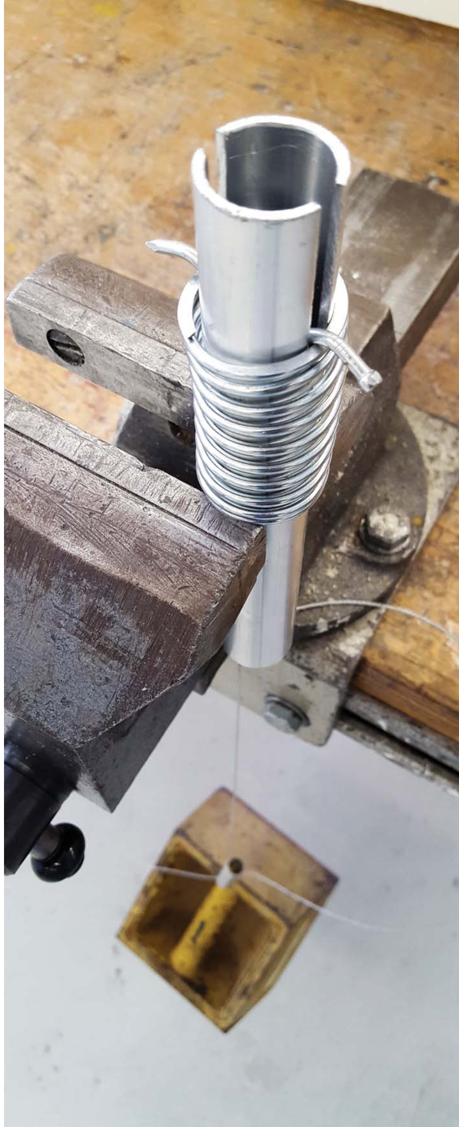
▶ Figure 41: Test set-up to validate the spring rate, consisting of an incised aluminium tube and a bent nail that moved in the incision.
