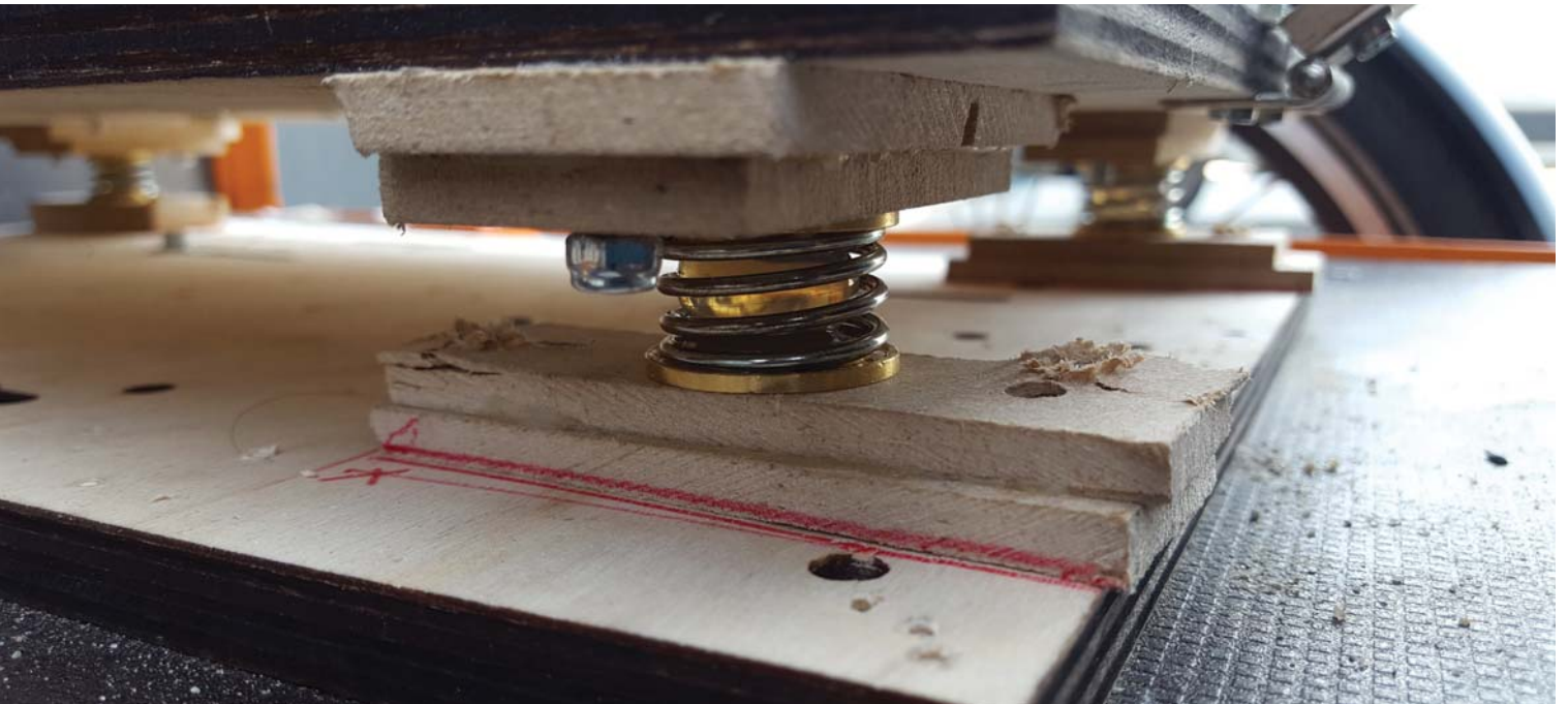
▲ Figure 49: This type of isolator used a coil spring together with a solidified silicone gel for damping.
