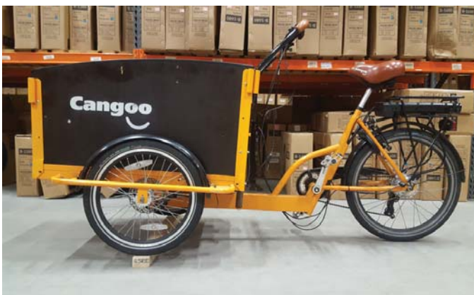
▲ Figure 101: To validate the natural frequency of both systems, the cargo bike was placed on top of a wooden beam with a height of 5 cm. A transducer was attached to the mechanism and the cargo bike was pushed backwards.
