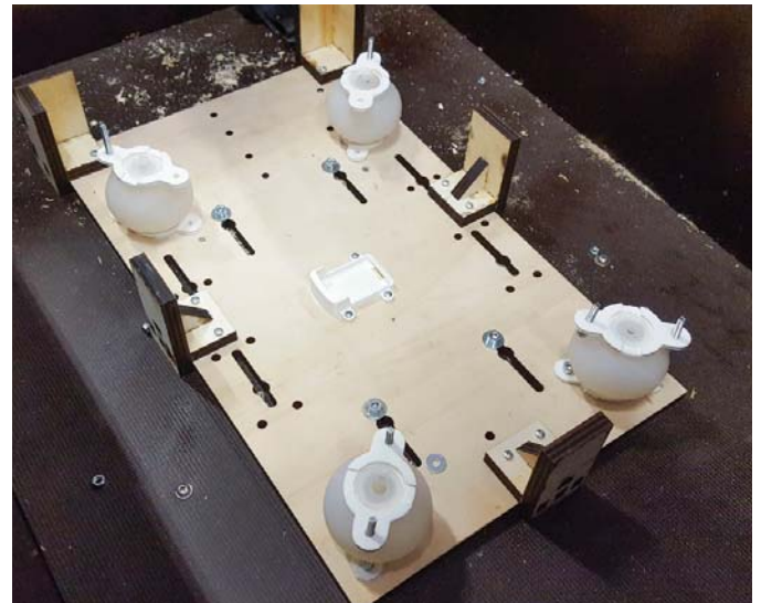
▲ Figure 46: Four rubber damping balls were placed at the corners of the platform construction. Inspiration was found from drones that use rubber damping balls to stabilize camera images
