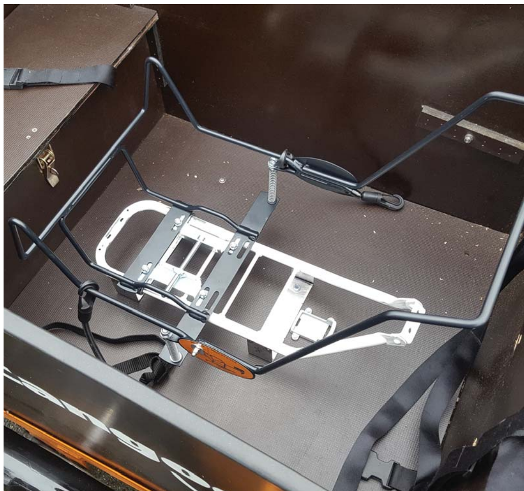
Figure 35: (Left) The Steco Baby Mee was installed on a special carrier that was anchored to the floor of the cargo bike.
