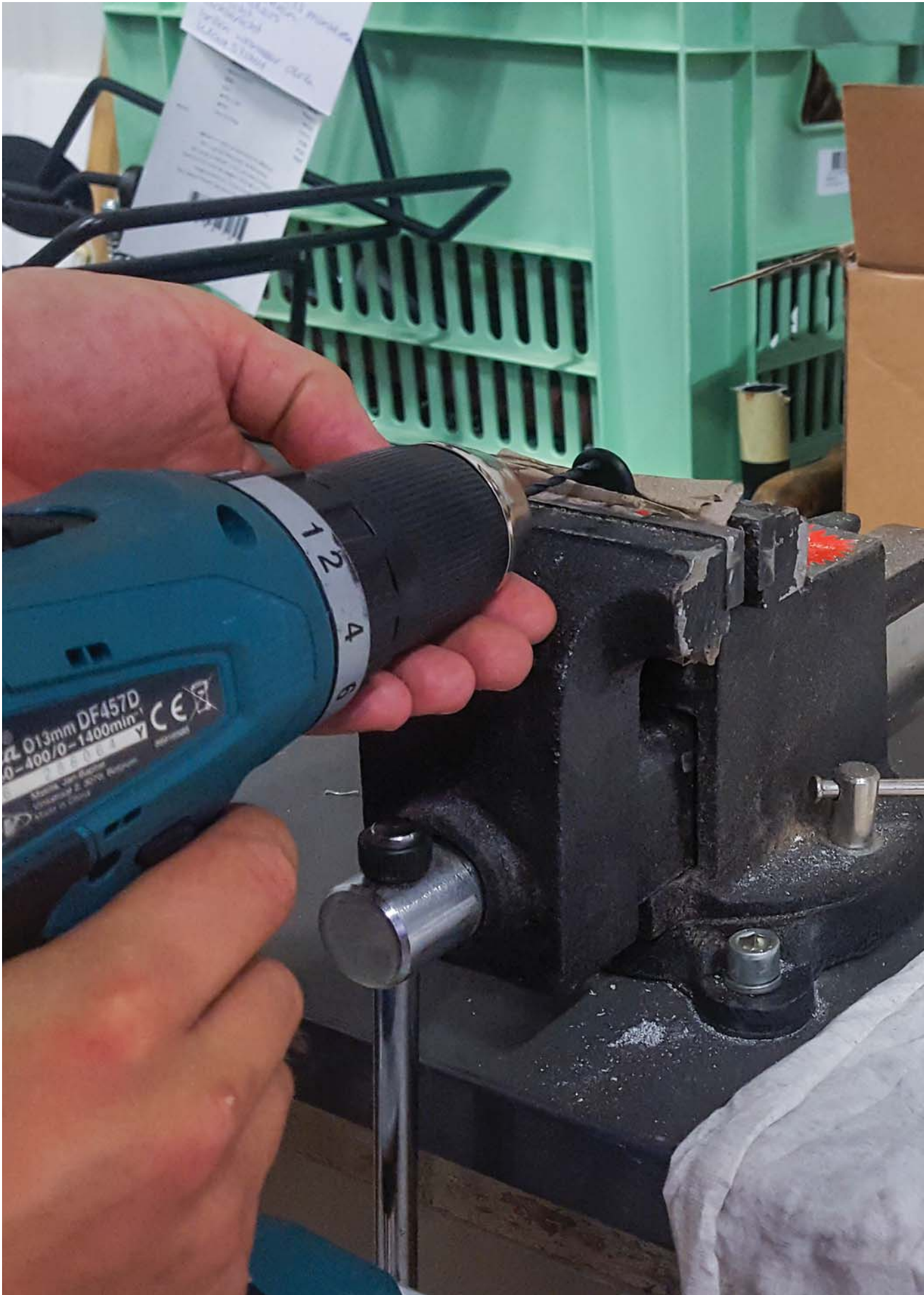
▲ Figure 58: In order to let the shock absorber react precisely to bumps in the road, both holes of the piston were drilled larger in steps of 0.5 mm after each test.
