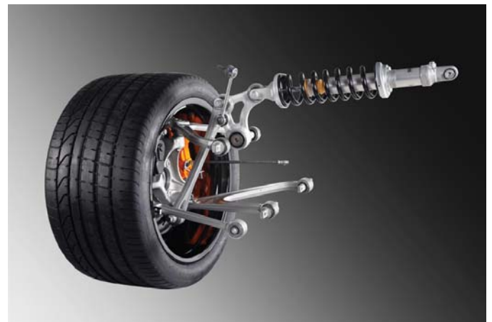
▲ Figure 60: Push rod suspension system of a Lamborghini Murcielago sports car
