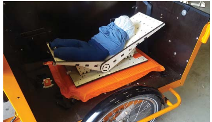
▲ Figure 50: An inflatable mat was cut and glued together to fit in the cargo bike. The inflatable mat was too unstable and wobbly.
