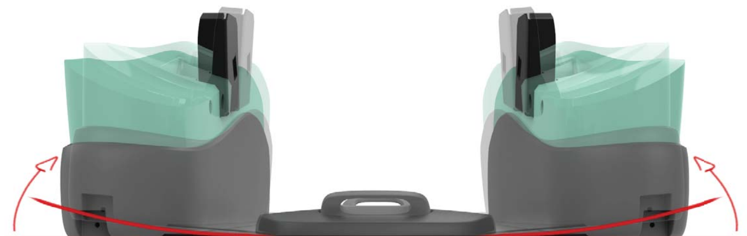
▲ Figure 82: Due to the little support on the side of the construction - the closure between the pins and the ground tile act in the middle of the construction - , the construction could 'flip'.
