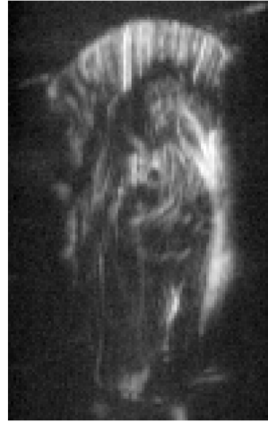
Figure B.4: Log of a single PDI illustrating the presence of sensor noise throughout scans as can be seen by the speckled effect in the dark regions of the image.
