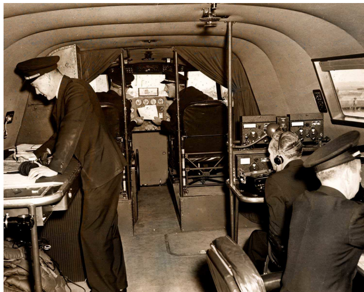
Figure 4-2: Five-crew Flight Deck of the Boeing 314 Clipper, courtesy of (luarelli, 2010)
