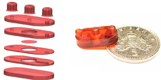
Figure 18. An exploded view rendering of the diaphragm pump is shown on the left and a photograph of the pump is shown on the right along with a UK 5 pence piece for scale. Adapted from: [121]
