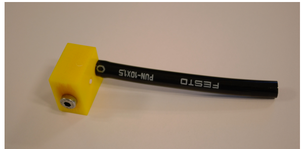
Figure 30. Photograph showing a sample from the first batch with the Festo tubing press fitted on the air connector.
