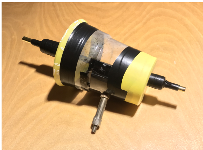
Figure 22. Photograph of the proof of principle prototype that was used to test if movement would be generated if the air chamber was sealed with two differently sized diaphragms.
