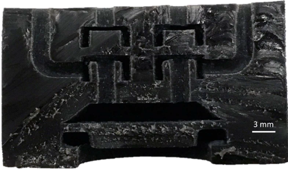
Figure 19. A photograph of the cross-section of the monolithic diaphragm pump, showing the three diaphragms inside. Adapted from: [122]
