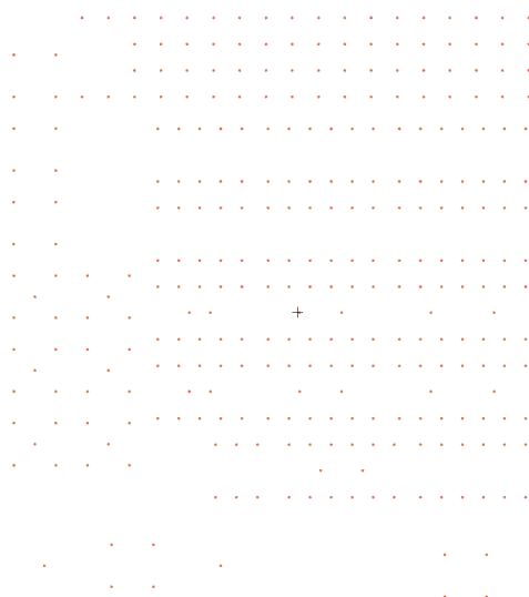
Figure A.3: Mask for CuNP pattern transfer with a diameter of 20 \mu\text{m}
