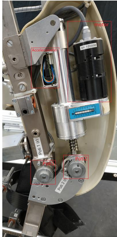
Fig. 9: Image of the inside of the knee actuator in the Lokomat® system. Source: HRI Wiki, TU Delft [4]
