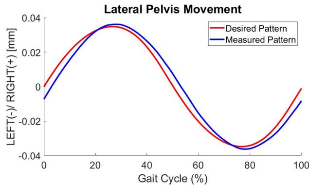
Fig. 16: Recordings of a subject showing slight actuator overshoot in the lateral pelvis movement trajectory compared to the desired trajectory.
