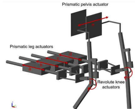
Fig. 2: Kinematic model of the modified Lokomat® in Simulink for gait pattern conversion. It includes four prismatic actuators for ad-/abduction and flexion/extension: (a) right outer, (b) right inner, (c) left inner, (d) left outer; one prismatic pelvis actuator (e) for lateral pelvis movement; and two revolute knee actuators (f) right and (g) left for knee flexion/extension.
