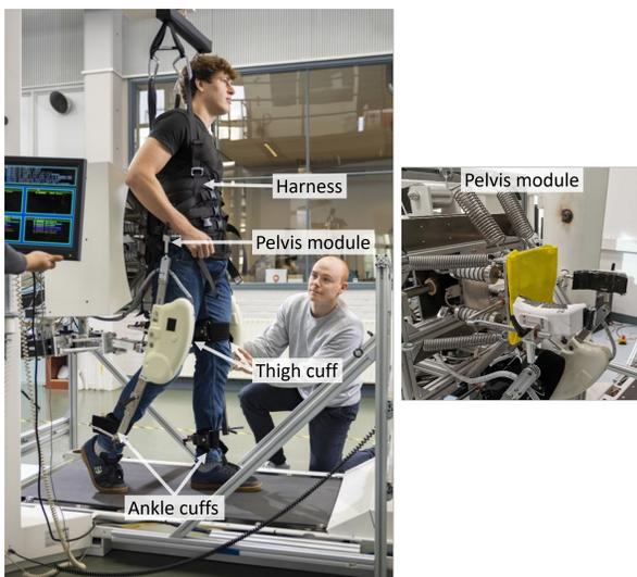
Fig. 1: Modified Lokomat® with a user secured, featuring ankle and thigh cuffs, a safety harness for fall prevention, and a pelvis module (right) with two banana-shaped supports for pelvis stabilization.
