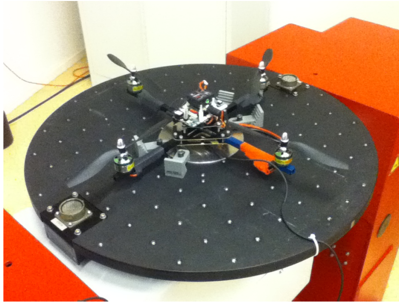
Figure 4-4: Quadrotor mounted on the turn table ready for testing
