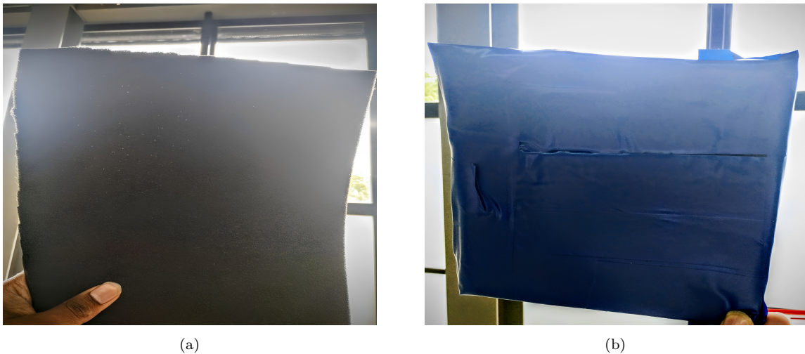
Figure 5.9: (a) The shading setup is not opaque because it has holes that let sunlight through. (b) The shading is covered with tape all around, and this tape helps attach the cover on top of the shaded cell using double-sided tape without causing any damage to the front surface.
